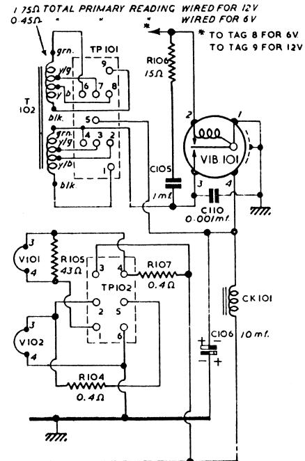
The circuit shown illustrates the valve heater and vibrator circuit arrangement for this unit. The remainder of the circuit is the same as that for model XA. Instructions regarding the conversion of the unit to either 6 or 12 volt operation may be found under Voltage Adjustment at the foot of the following page.
