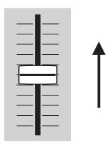
the sound volume is too low, adjust the GAIN fader no.6 to a point were the LED meter on the side reaches orange.
