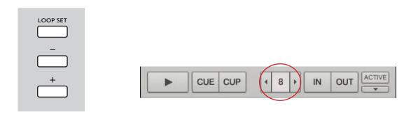
+/- The length of the loop is adjusted with the button. The current length is shown in each deck.
