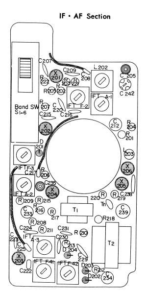
♣ Parts to be mounted on the printed side : L206, C243, R223, R224, R225, C237, C240, C241 C236, C245
