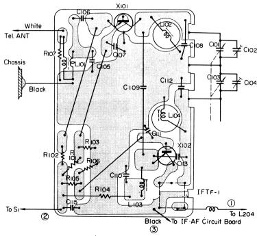
C113 is mounted on the printed side.
