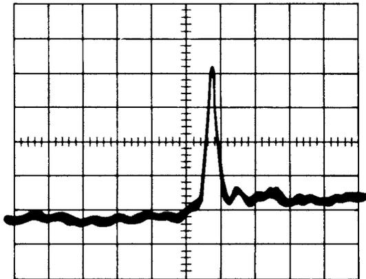
adjust the GAIN control so that the open end display (reflected pulse) is set 2 divisions above the cable display (horizontal centerline). This sets the reflected pulse to  $+1\rho$  from the characteristic impedance.
