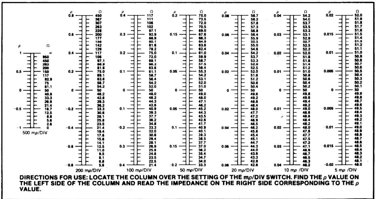
Figure 2-8. Impedance nomograph
