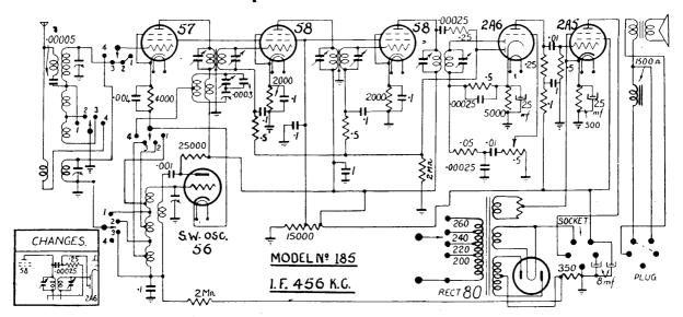
Tasma model 185 is a seven-valve receiver designed for "all-wave" coverage (four bands—13/27, 25/50, 48/100 metres, (four bands—13/27, 25/50, 48/100 metres, and broadcast) and operation from 200-260 volts A.C. mains. This receiver is of the console type and is fitted with four controls, these being for volume, tuning, wave-change and aerial circuit trimming (on short-wave bands only). The loudspeaker fitted is an eight-inch unit with a field-coil resistance of 1,500 ohms.
