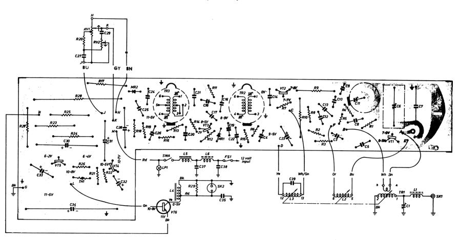
Notes: The diagram represents the view from the wiring side of the printed board.
