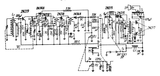
Circuit diagram of right channel (Left channel is the same as above except 200 $\mu$  F. M. CH, Battery)
