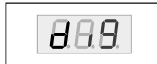
Figure 2-1 7-segment example, entering diagnostics
