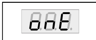
Figure 2-2 7-segment example, diagnostic main menu
