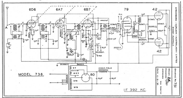
Stromberg-Carlson model "736" is a seven-valve dual-wave receiver. Coverage on the "broadcast" band is from 195 metres to 570 metres, thus allowing a reasonable percentage of margin at each of the bands. Short-wave coverage is from 16.8 to 51 metres. This receiver is of the console type and is fitted with four controls, as shown on the accompanying top-chassis layout.
