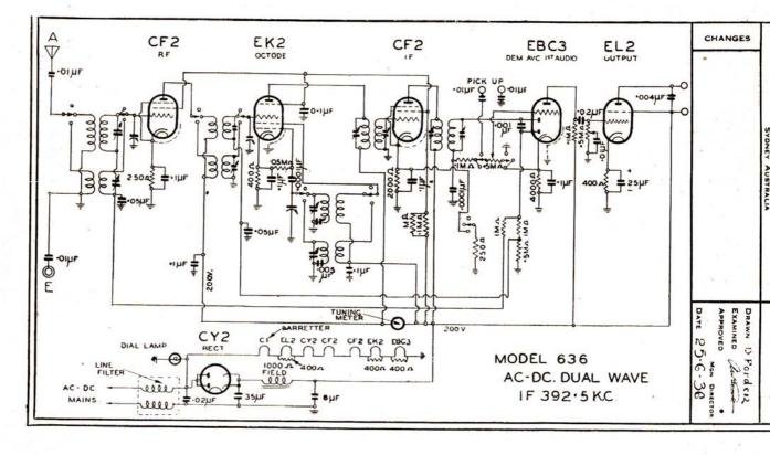
TROMBERG-Carlson Model 636 is an A.C.—D.C. six valve superheter-odyne, using Philips valves, which include the current limiting "Barretter" in place of a ballast resistor. The inclusion of this barretter enables the receiver to be used on any supply between 160 and 260 volts without the necessity for any adjustment.
