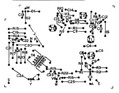
DO NOT USE: AN IRON OVER 60W-EXCESS SOLDER-UNDUE PRESSURE, REPLACE COMPONENTS BY-WITHDRAWING SOLDER FROM THE CRIMPED LEADS WHILE LIFTING THE LEAD FROM THE FOIL BY THE INSERTION OF A KNIFE EDGE. CUT OFF THE CRIMPED SECTION AND WITHDRAW COMPONENT. OR-CUT OUT COMPONENT, UNSOLDER REMAINING TERMINATIONS AND PUSH THROUGH. REPAIR FOIL BREAKS BY: FLOWING SOLDER, OR SOLDERING TINNED COPPER WIRE ACROSS. REPLACE DAMAGED SECTIONS WITH A JUMPER OF WIRE.
