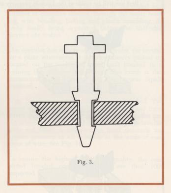
For printed boards of  $\frac{1}{16}$ " thickness board hole size should be 1.3mm (0.051"), and shoulders A and B act as buffer and lock. Fig. (4).
