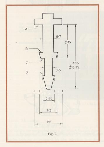
For printed boards of 1mm thickness board hole size should be 0.8mm (0.031"), and shoulders C and D act as buffer and lock respectively. Fig. (3).
