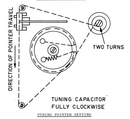
Set tuning capacitor to closed position, i.e., fully anti-clockwise. Slide pointer carriage along cord so that edge of carriage and dial background align as indicated in diagram. Crimp lugs on pointer carriage to dial cord.
