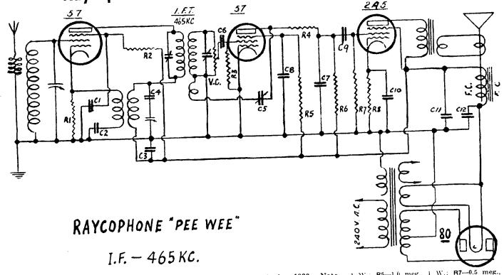
The Raycophone "Pee-Wee" is a fourvalve midget receiver designed for broadcast coverage and operation from A.C. mains. This receiver uses a compact speaker with a field-coil resistance of 2,500 ohms. Two panel controls are fitted for volume control and tuning and.
