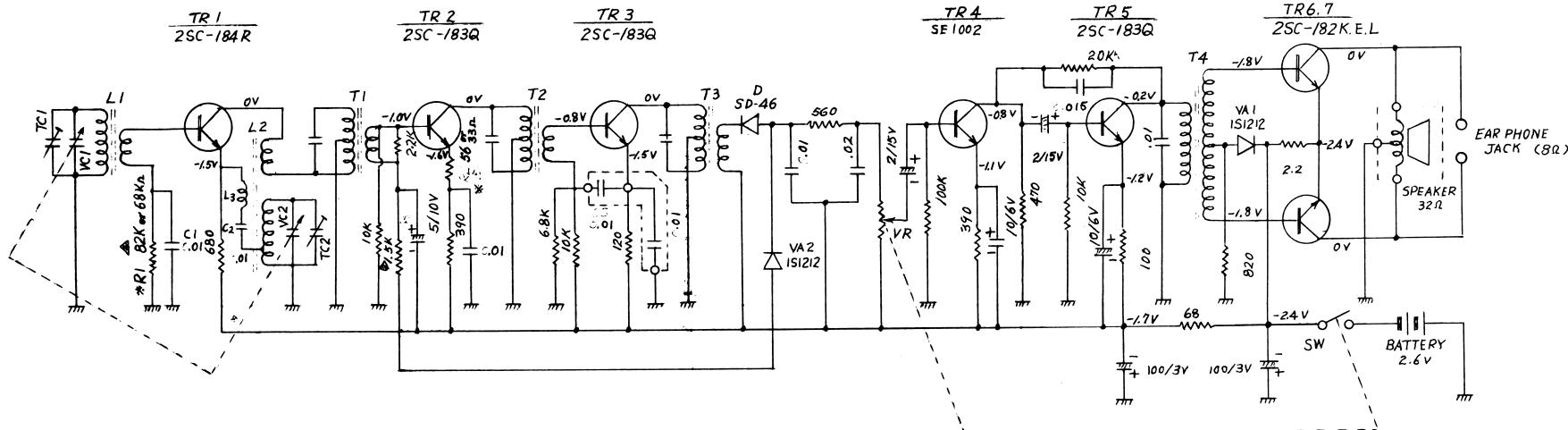
Voltages shown in this diagram indicate values, which measured under supply voltage of 2.6volts (capable .500mA current drain) with a 4.4ohms resistor in series and volume control at minimum level.
