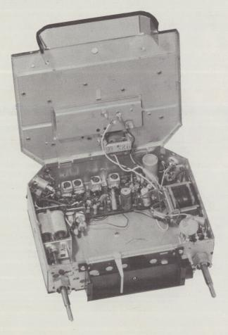
Tuning Range: Intermediate Frequency: 455 KHz Supply Voltage: 13.0 Volts D.C. Current Consumption: 650 MilliAmps Power Output: Speaker Impedance:
