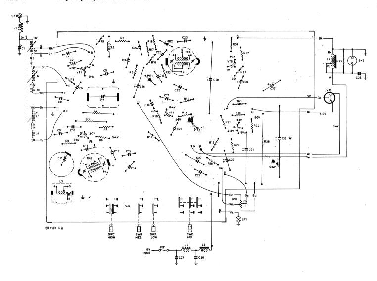
All voltages shown are positive with respect to the board earth, and are measured with no signal input and volume maximum clockwise using a 20,000 ohm/volt meter. Blue indicates the printed wiring.
