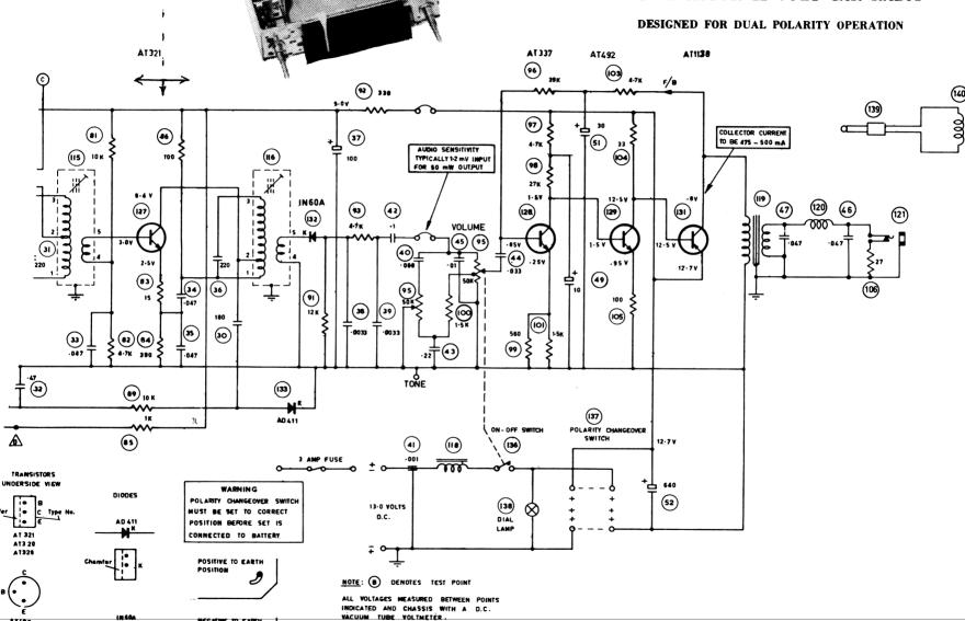
NUMBERS ASSIGNED TO TERMINALS OF COILS AND TRANSFORMERS ARE TO FACILITATE POLARITY CHANGEOVER SWITCH CIRCUIT TRACING AND COMPONENT REPLACEMENT AND MAY NOT BE FOUND ON THE UNIT.
