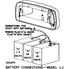
Instructions for Connecting Heavy Duty External Batteries.
