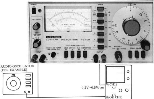
Fig. 2-4 Scope connections.
