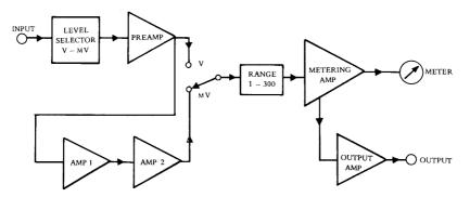
Fig. 3-6 Simplified block diagram for voltage measurement.
