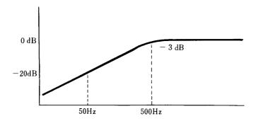
Fig. 3-7 High-pass filter characteristic.
