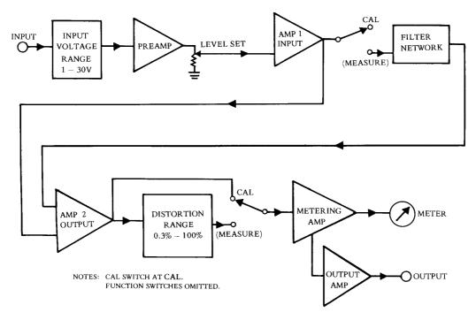
Fig. 3-3 Distortion measurement: Simplified block diagram.
