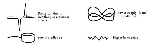
Fig. 2-7 Distortion observed with Lissajous patterns.
