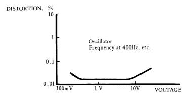
Fig. 2-8 A: Output VS. distortion.
