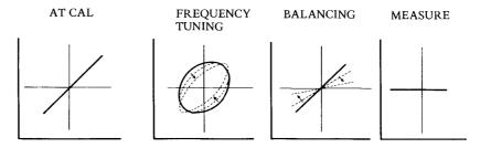
Fig. 2-6 Using the Lissajous pattern.
