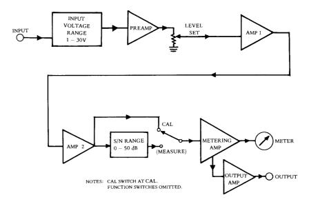
Fig. 3-5 Simplified block diagram for S/N measurement.
