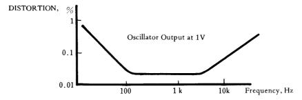
Fig. 2-8 B: Frequency VS. distortion.
