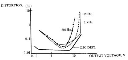
Fig. 2-9 A: Amplifier output VS. distortion.
