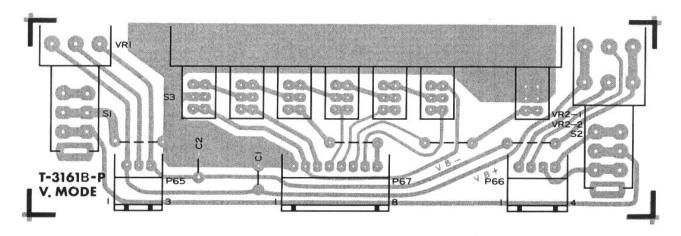
Figure 5-17 LBO-516 Vertical Mode P.C. Board T-3161B
