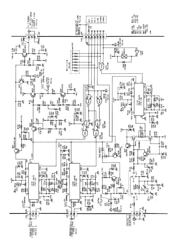
Figure 5-5. LBO-516 CH-3 Input Circuits and A Time-Base Trigger Source Switching
