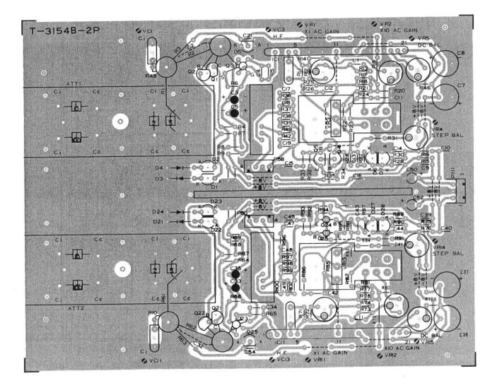
Figure 5-15. LBO-516 Vertical Input Attenuator and Amplifier P.C. Board T-3154B
