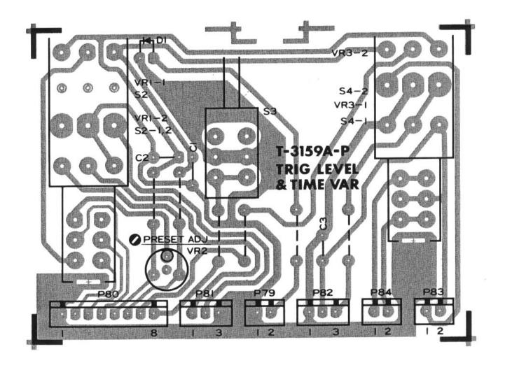
Figure 5-19 LBO-516 Trigger Level and Time Variable P.C. Board T-3159A
