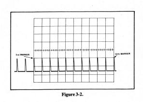
the time-mark generator to 0.5 S and connect it to the CH- 1 input connector. Align the first mark with the left-most vertical graticule line. Adjust the generator so that each subsequent mark is aligned with a major vertical graticule line. Repeat for each A TIME/DIV switch setting from.2 S to 0.2 $\mu$ S, verifying that the timebase accuracy is within +-2% at each sweep speed.
