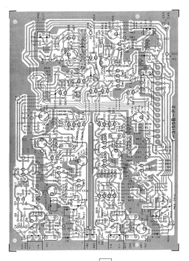
Figure 5-16. LBO-516 Vertical Preamplifier P.C. Board T-3155B
