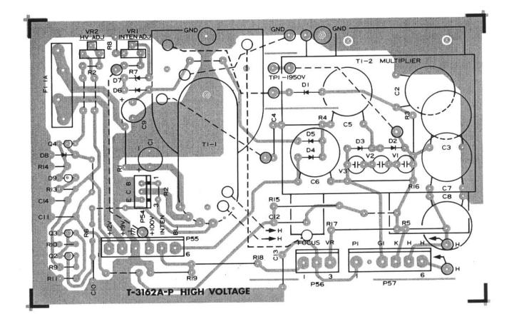
Figure 5-23 LBO-516 High Voltage Oscillator P.C. Board T-3162A
