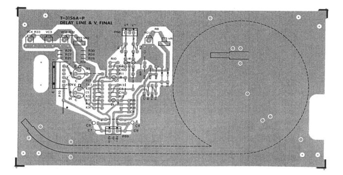
Figure 5-18 LBO-516 Delay Line and Vertical Final Drive P.C. Board T-3156A
