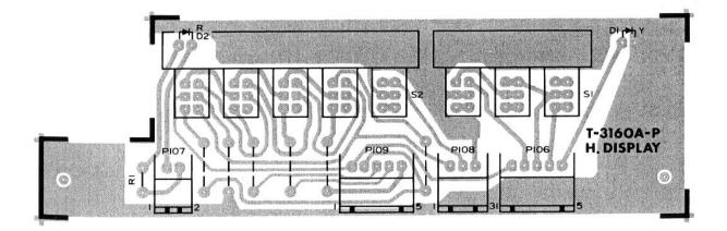
Figure 5-22 LBO-516 Horizontal Display P.C. Board T-3160A
