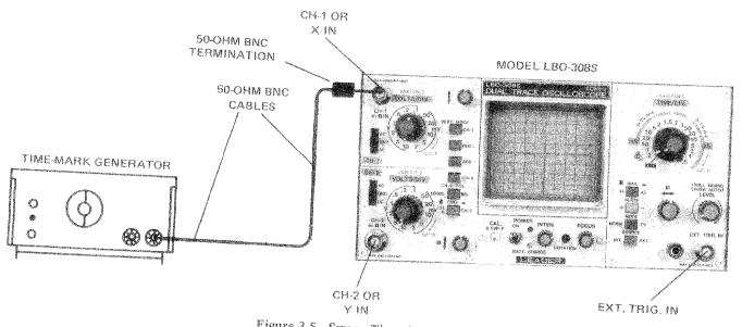
Figure 3-5. Sweep Time Accuracy Test Setup
