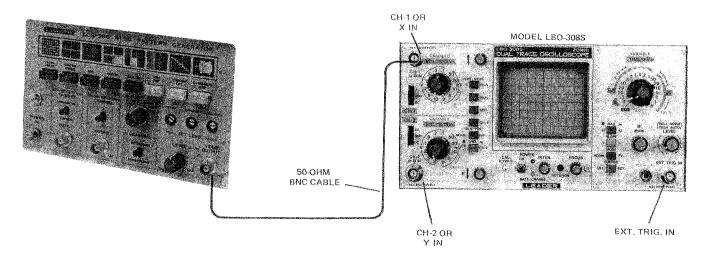
Figure 3-6. TV Sync Triggering Test Setup
