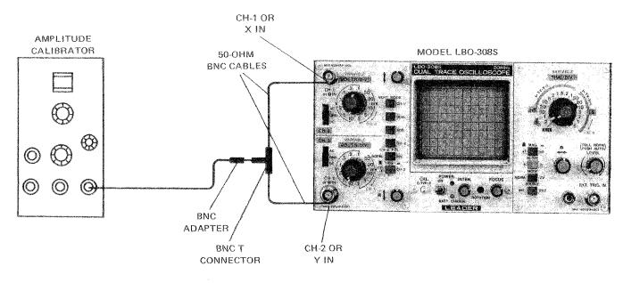
Figure 3-1. Deflection Accuracy Test Setup
