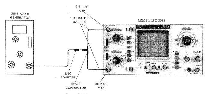
Figure 3-7. Phase Measurement Test Setup
