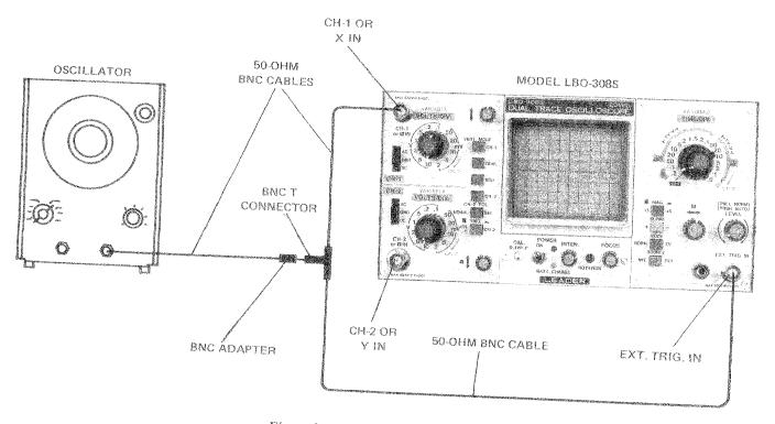
Figure 3-3. 50-Hz Triggering Test Setup
