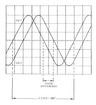
Figure 2-14. Dual-trace Method of Phase Measurement
