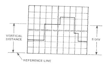
Figure 2-10. Instantaneous Voltage Measurement
