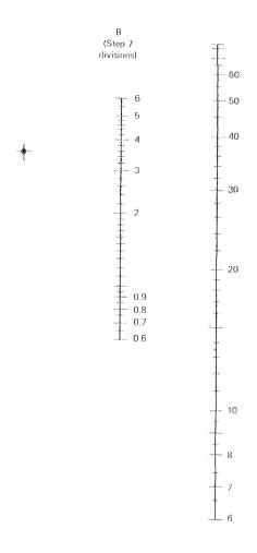
Figure 2-16. Phase Angle Nomograph
