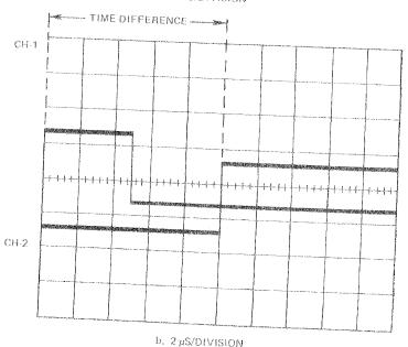
Figure 2-13. Measuring Lead and Lag Time
