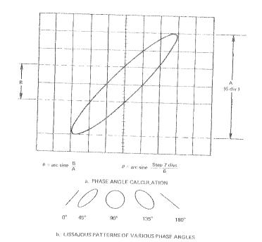
Figure 2-15. Lissajous Method of Phase Measurement
