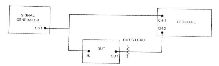
Figure 2-17. Test Setup for Distortion Comparison and Phase Measurement.
