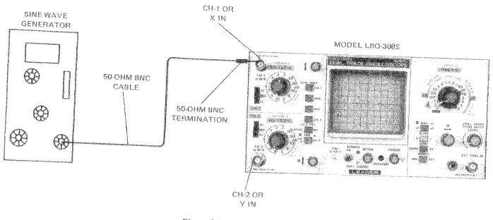
Figure 3-2. Bandwidth Test Setup
