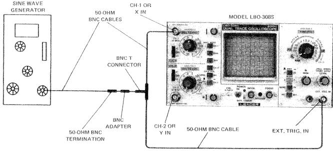
Figure 3-4. 20 MHz Triggering Test Setup
