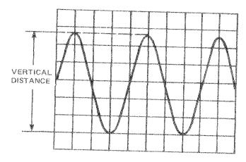
Figure 2-9. Peak-to-peak Voltage Measurement
