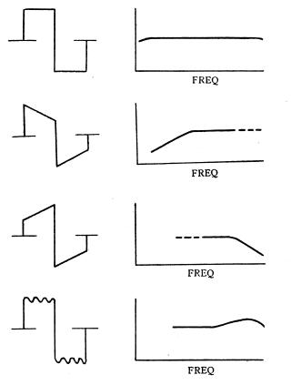
Low gain at low freq. Insufficient L in output transformer; grid coupling capacitors too small
