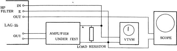
Fig. 5 IM DISTORTION TEST SET-UP
