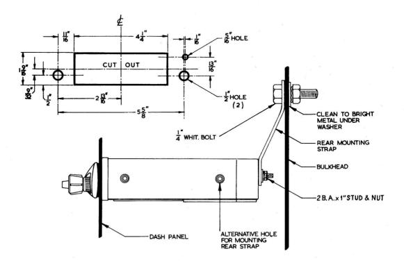
FIG. 2 RECEIVER MOUNTING IN DASH PANEL
