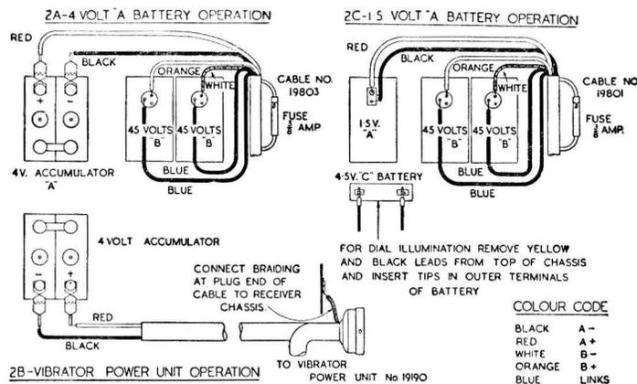
FIG. 2 - BATTERY CONNECTIONS 20380
