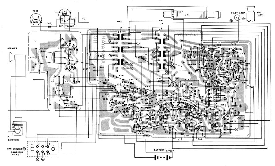
SW-1 A, B, C, D, E, F shown FM position. SW-2 A, B, C, D, E, F shown portable rodio use position.
