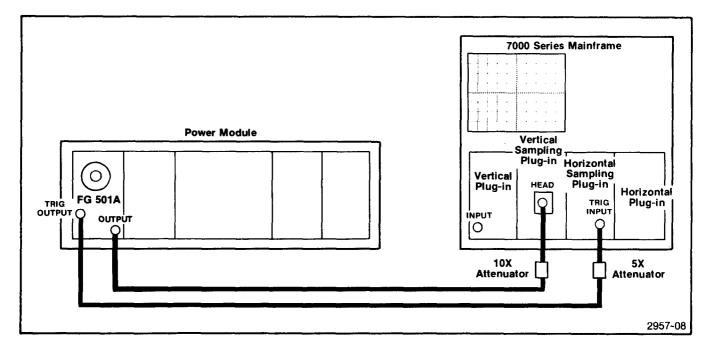
Fig. 4-4. Test setup for SQUAREWAVE COMP/RISE and FALL TIME adjustments.
