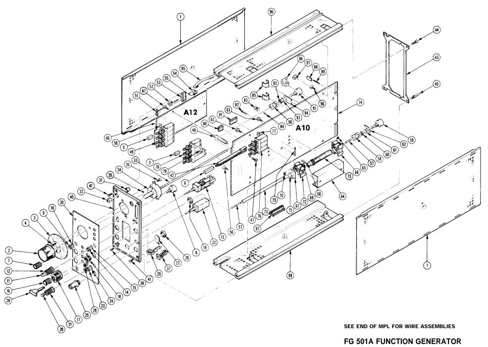
**FG 501A FUNCTION GENERATOR EXPLODED VIEW**
