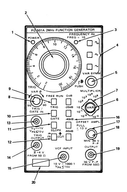
Fig. 2-2. Controls and connectors.
