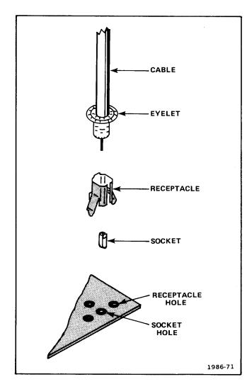
Fig. 5-1. Coaxial end lead connector assembly.
