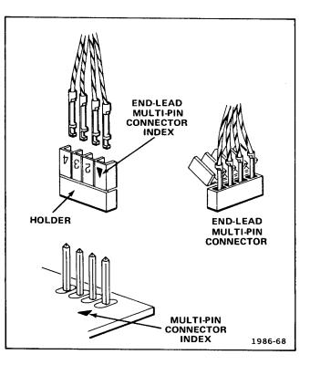
Fig. 5-2. Orientation and disassembly of multipin connectors.
