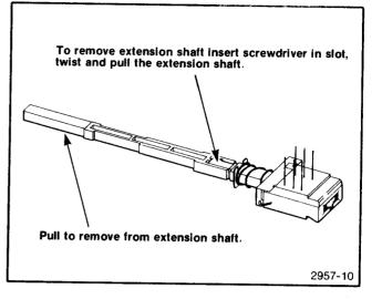
Fig. 5-3. Extension shaft and pushbutton removal.
