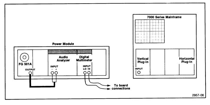
Fig. 4-2. Test setup for SINE DISTORTION adjustment.
