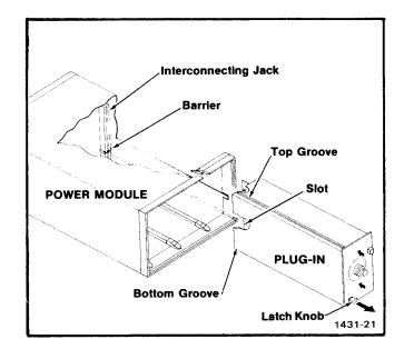
Fig. 2-1. Plug-in installation and removal.
