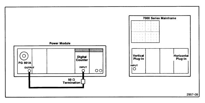
Fig. 4-5. Test setup for DIAL CAL and LOOP DELAY adjustments.
