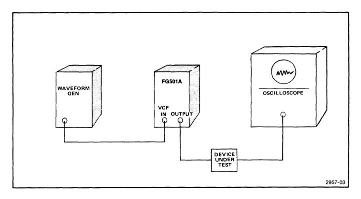
Fig. 2-11. Analyzing circuit or system response.
