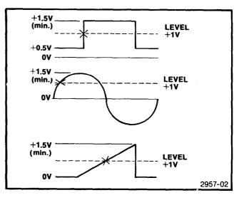
Fig. 2-7. Trigger Signal amplitude requirements and triggering points.
