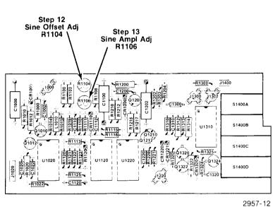
Fig. 8-1. Auxiliary Board.
