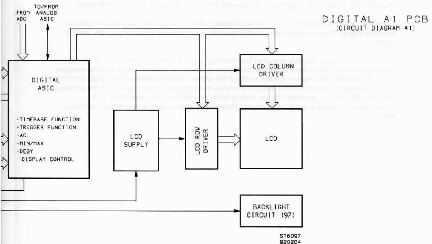
Figure 3.2 Block diagram main parts digital circuitry
