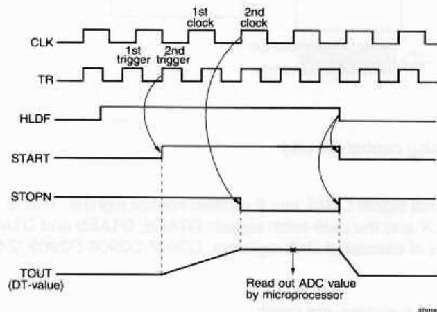
START: internal (in the A-ASIC) start signal for the Delta-T measurement.
