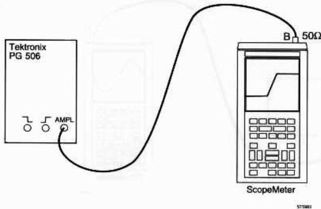
**Procedure for channel B rise time measurement:**
