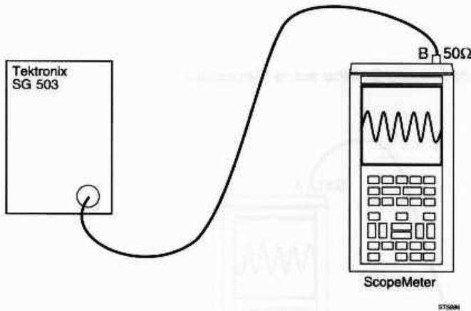
**Procedure/requirements for channel B trigger sensitivity measurement:**
