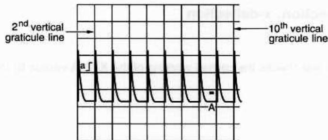
**Figure 4.6** The distance between the 10<sup>th</sup> marker pulse and the 10<sup>th</sup> vertical grid line must be the same as the distance between the 2<sup>nd</sup> marker pulse and the 2<sup>nd</sup> vertical grid line.
