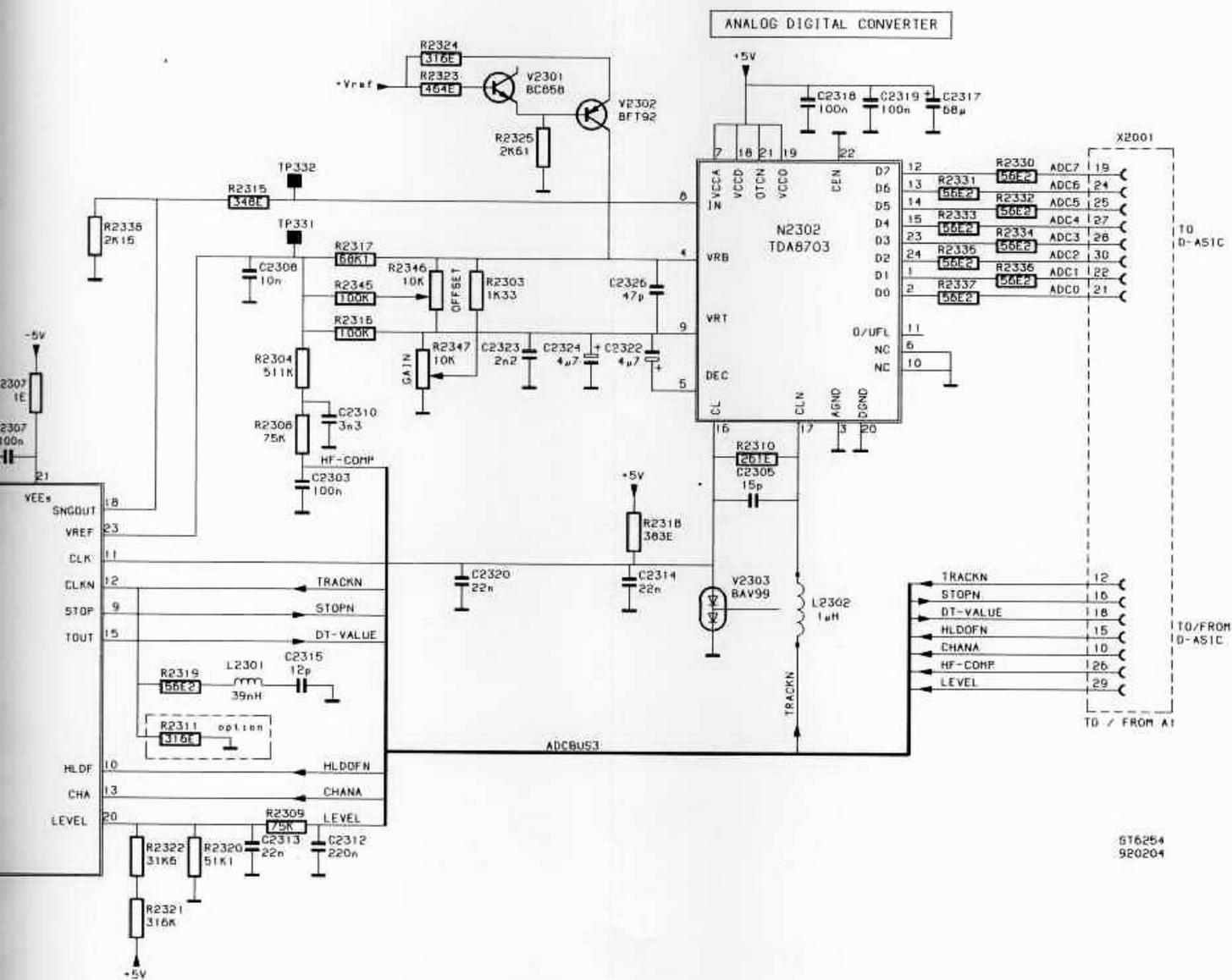
Figure 10.5 Analog A2 circuit diagram A2a
