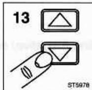
D Without changing the amplitude of the sine wave signal, switch over to step 13 using the upper select/adjust key. Increase the frequency of the sine wave to 50 MHz and check that the vertical deflection is 4.2 divisions or more.
