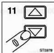
B Without changing the amplitude of the sine wave signal, switch over to step 11 using the upper select/adjust key. Increase the frequency of the sine wave to 50 MHz and verify that the vertical deflection is 4.2 divisions or more.
