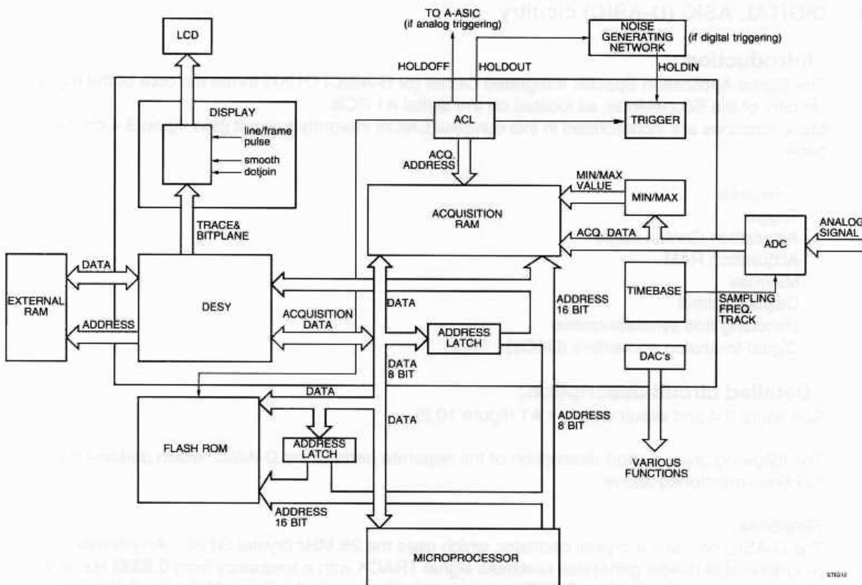
Figure 3.4 Schematic Diagram D-ASIC D1203
