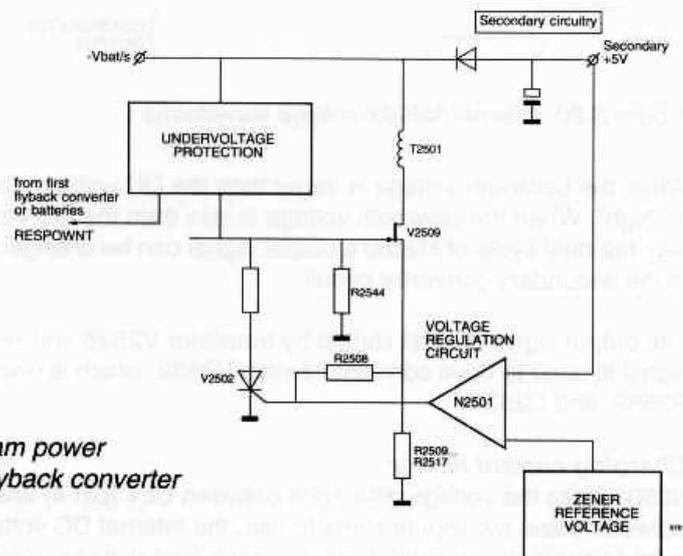
Figure 3.21 Schematic diagram power supply, second flyback converter
