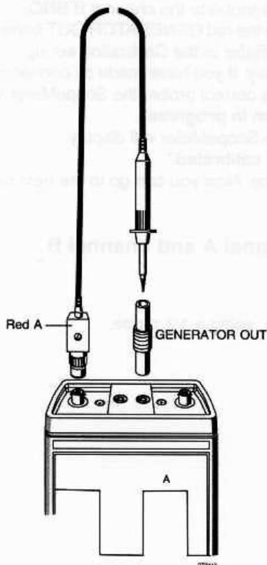
**IMPORTANT:** Calibration steps M19 and M20 determine the internal calibration constants that compensate for probe characteristics. To achieve full accuracy (as listed in the specifications in chapter 2), calibrations M19 and M20 must be performed, using the probes that are normally to be used with the instrument.
