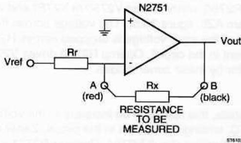
Figure 3.11 Ohm measurement circuitry (principle of operation)
