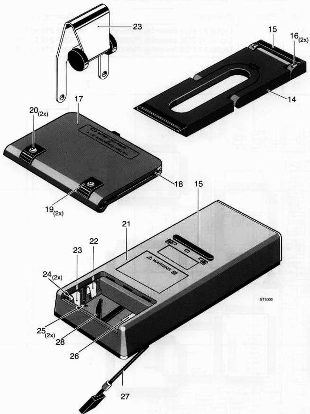
Figure 9.3 Battery contact assembly
