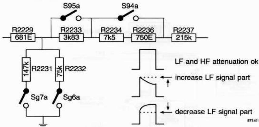
Figure 3.9 Automatic adjustment of the L.F. attenuation
