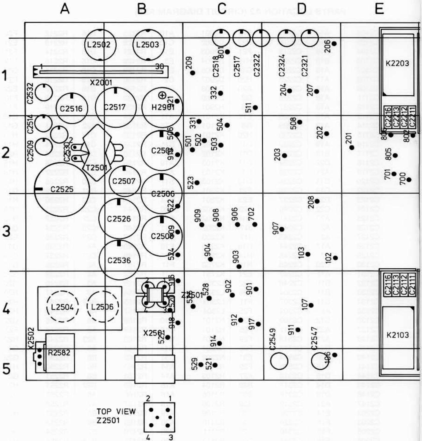
Figure 10.4 Analog A2 PCB (wired component side)
