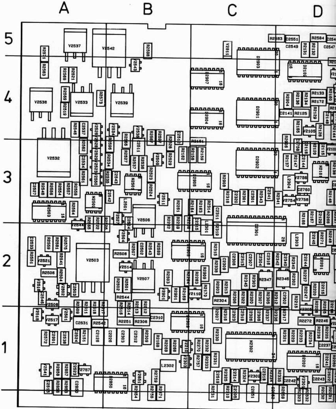
Figure 10.3a Analog A2 PCB (SMD components side)
