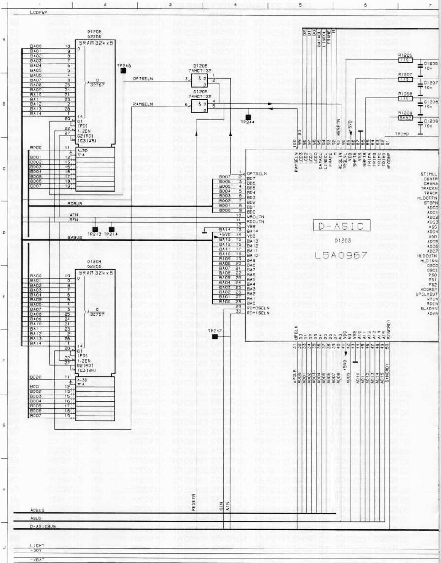
Figure 10.2b Digital A1 circuit diagram (part b)
