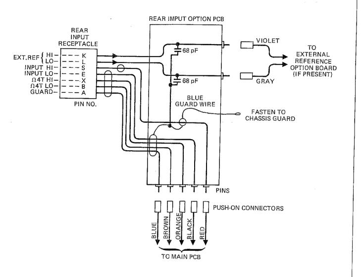
Figure 8-14. Rear Input PCB Assembly, Option -006
