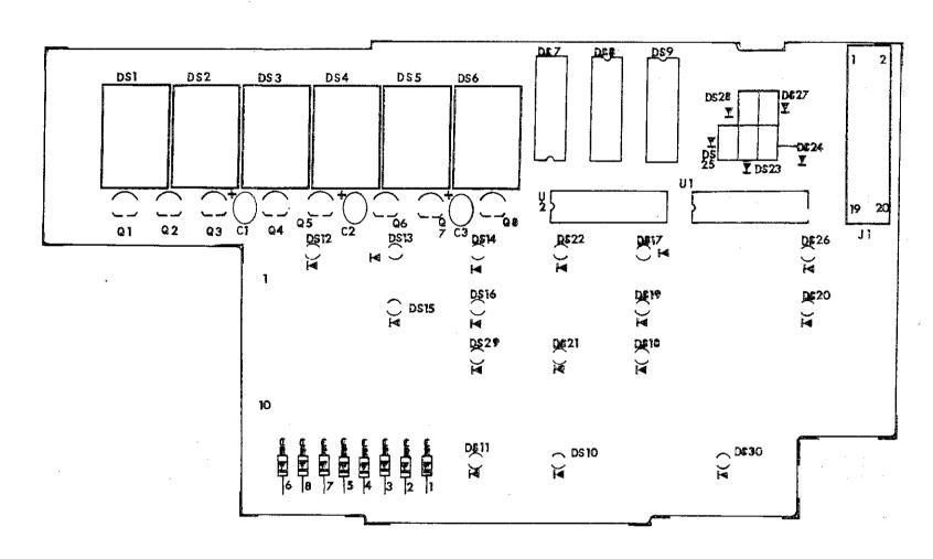
Figure 8-4. A2 Display PCB Assembly
