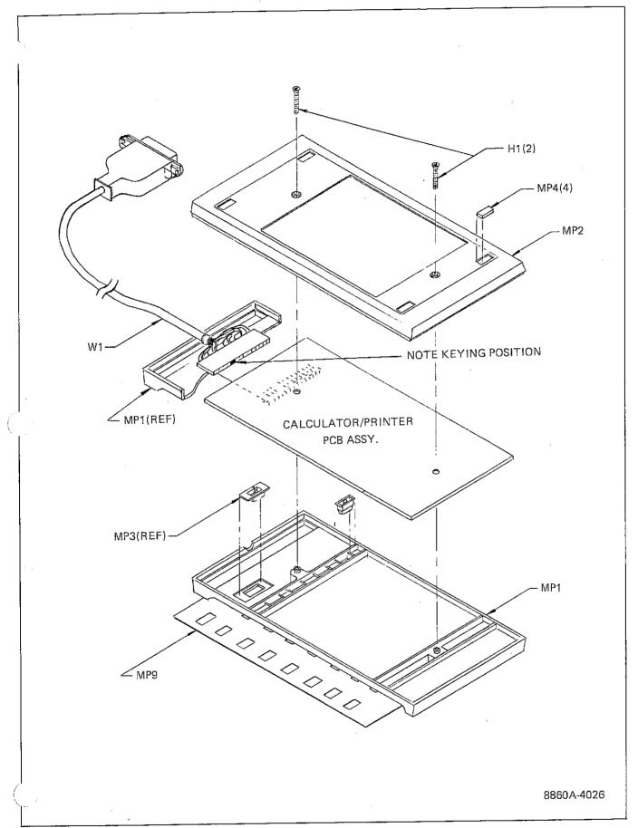
Figure 004-3. Control Keyboard PCB Assembly (cont)
