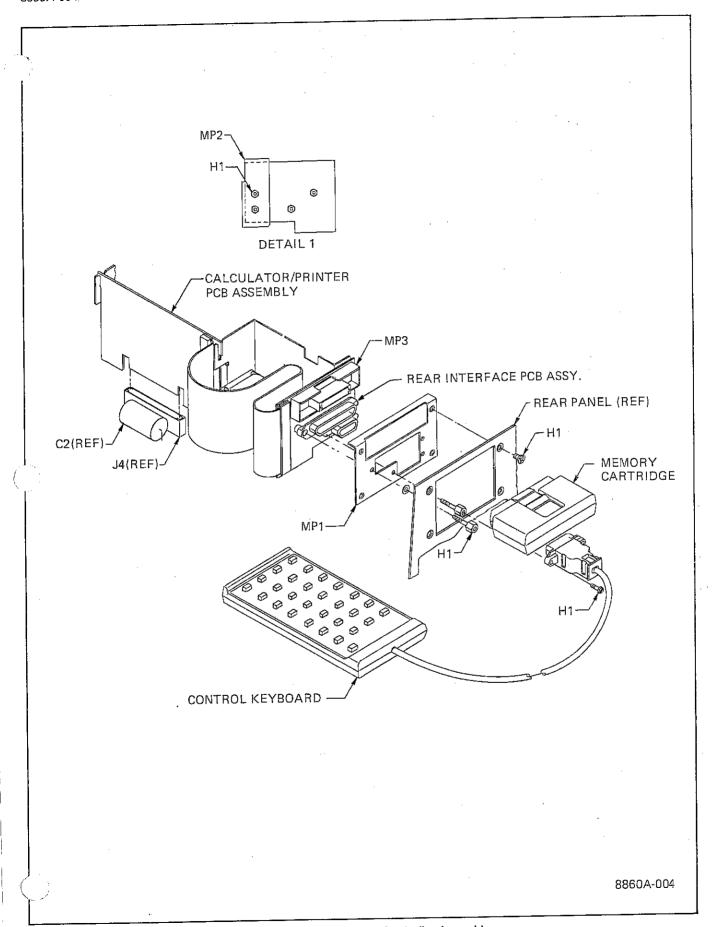
Figure 004-2. Calculating Controller Assembly
