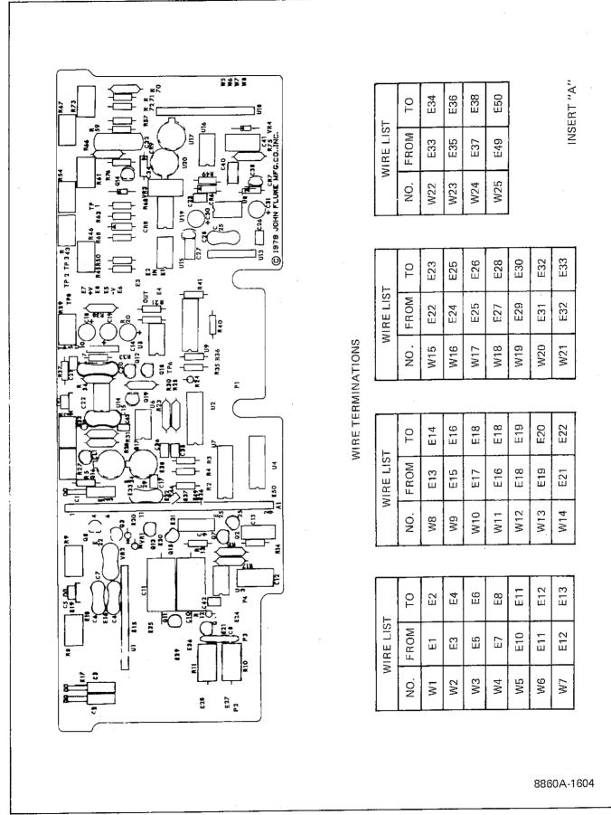
Figure 5-5. A4 AC/DC Scaling PCB Assembly
