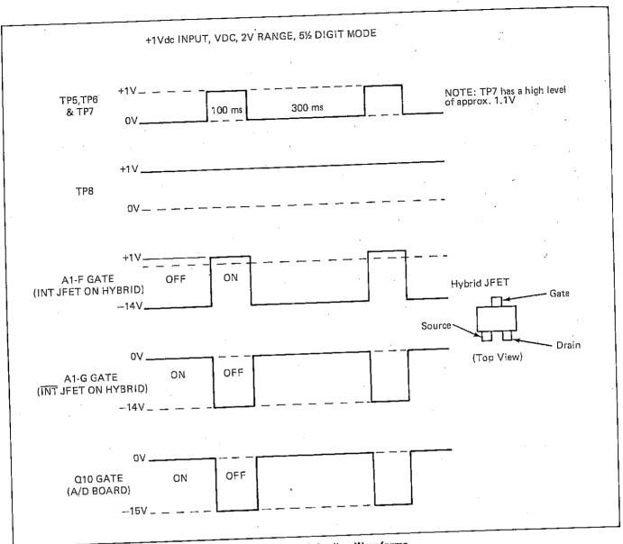
Figure 4-3. AC/DC Scaling Waveforms
