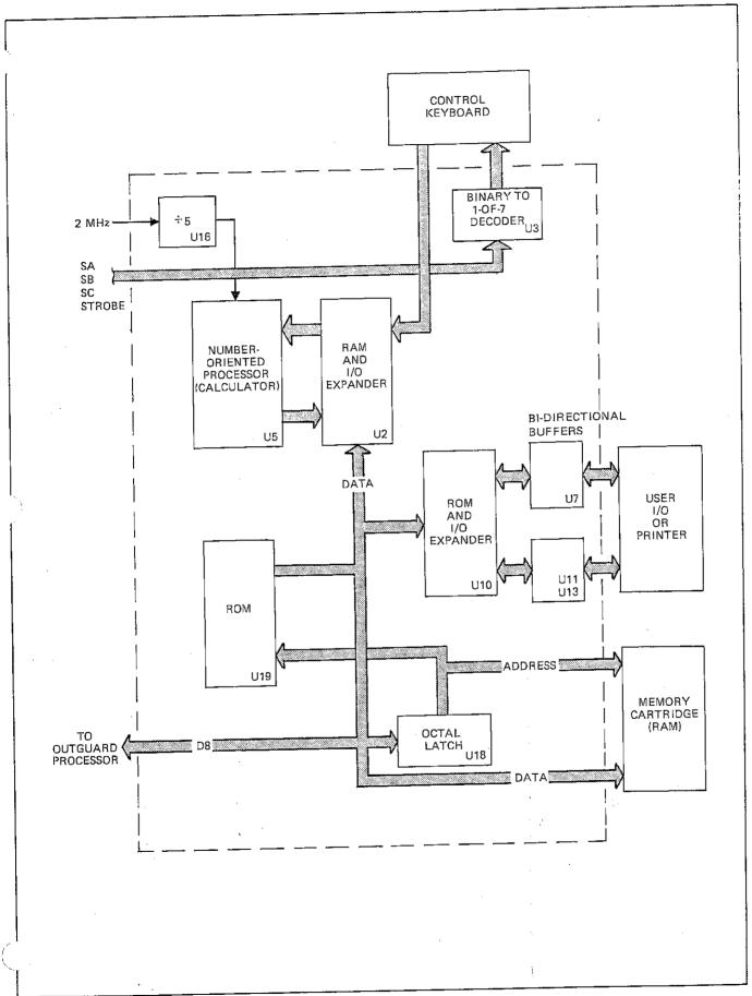
Figure 004-1. Calculating Controller Option-004 Block Diagram
