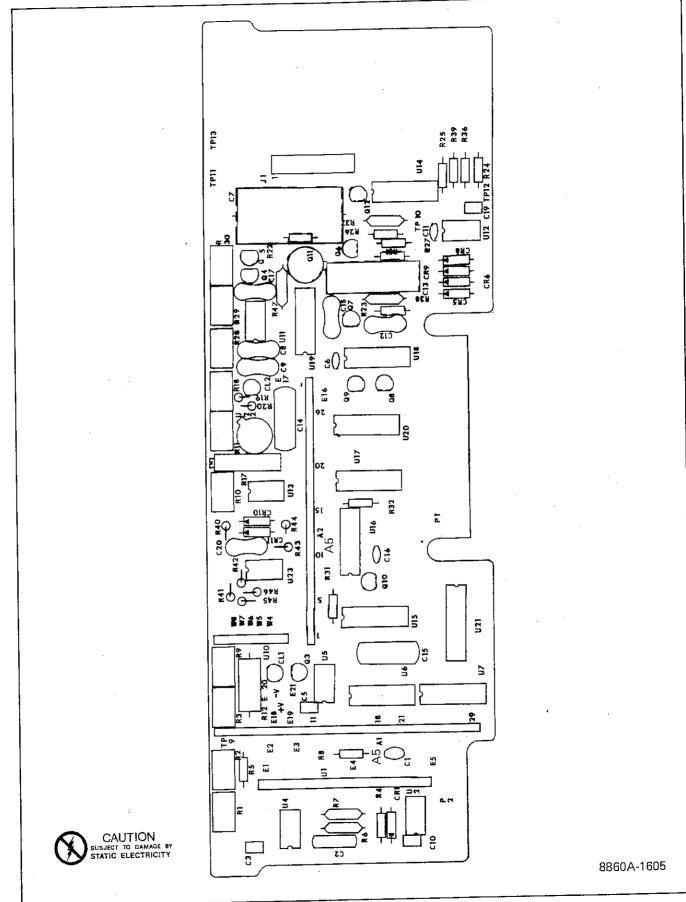
Figure 5-6. A5 A/D and Ohms Converter PCB Assembly
