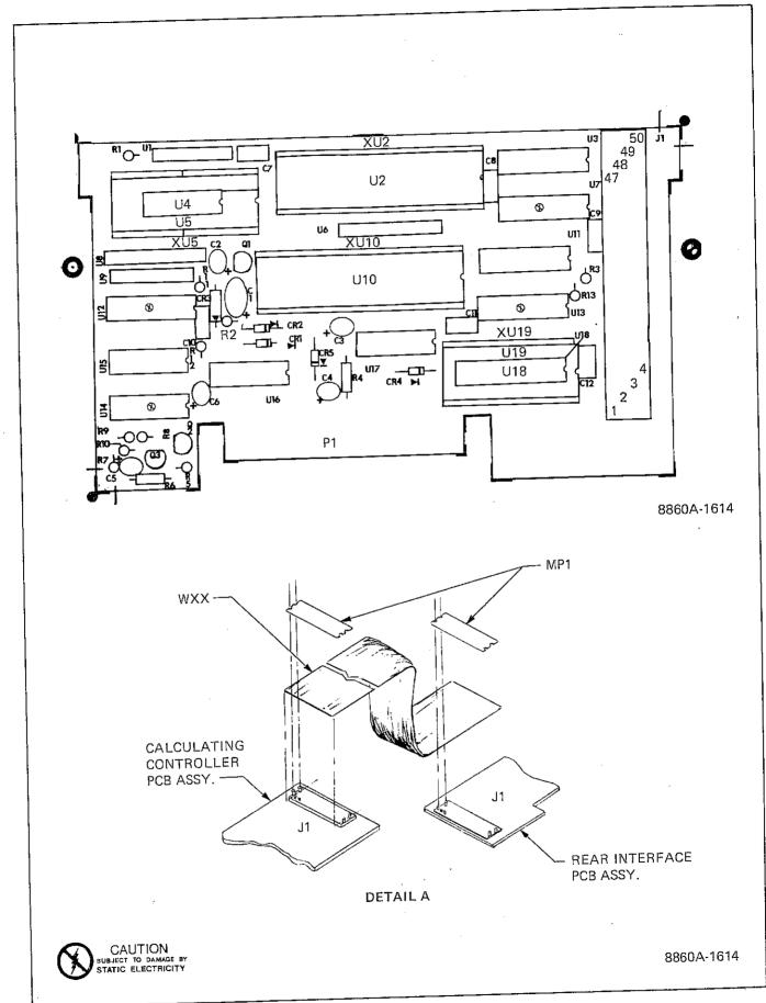
Figure 004-5. Calculator/Printer PCB Assembly
