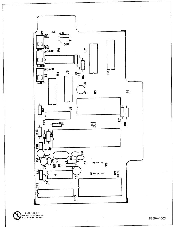
Figure 5-4. A3 Controller PCB Assembly
