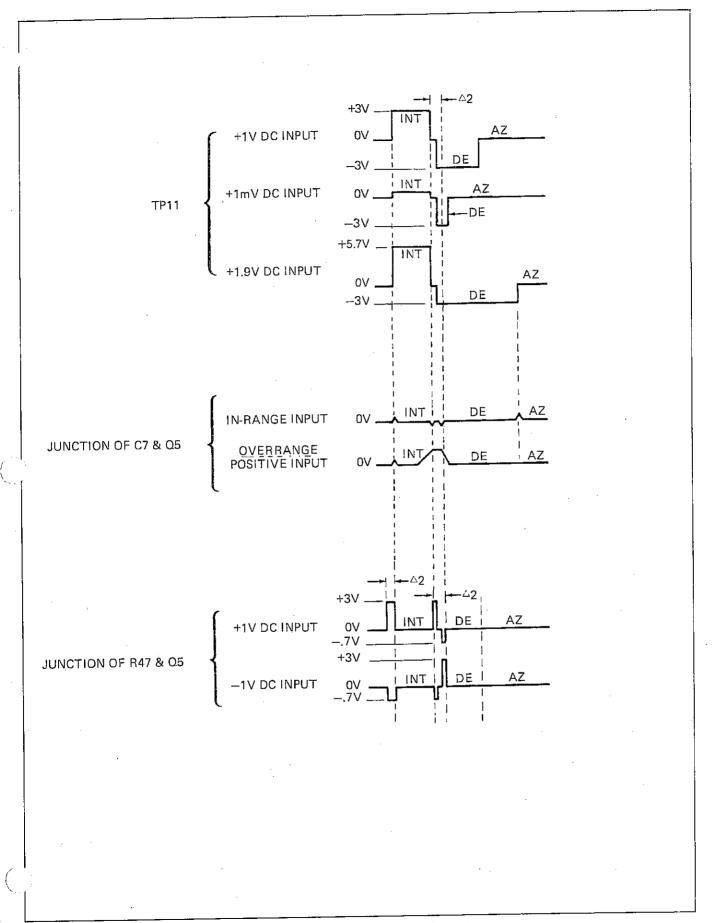
Figure 4-5. Signal Waveforms in A/D Converter
