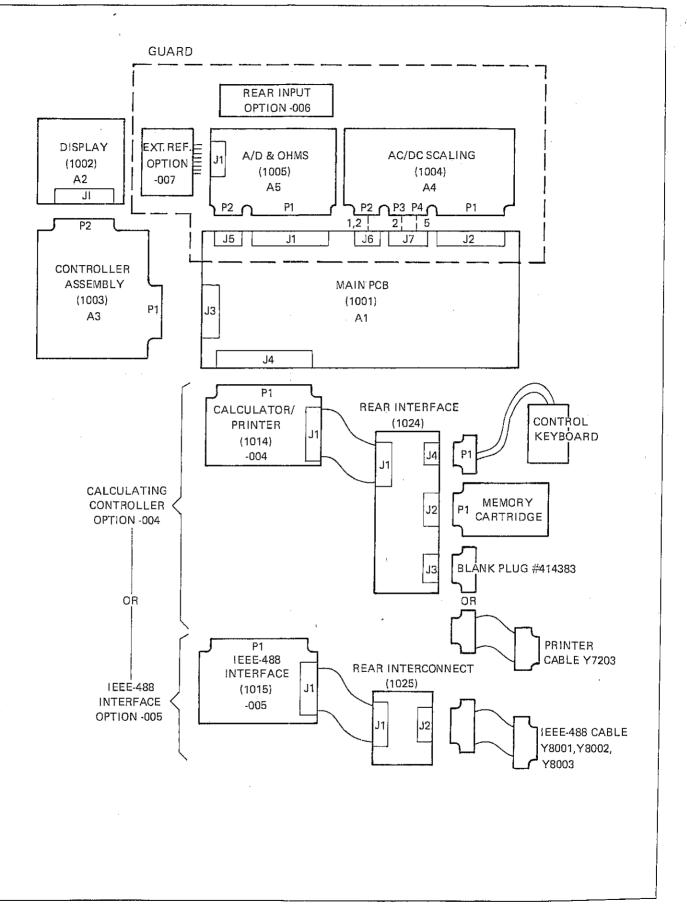
Figure 8-2, 8860A PCB Interconnect Diagram
