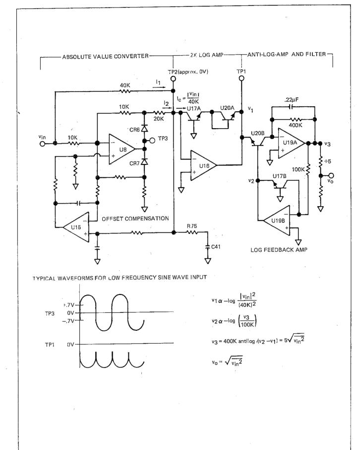
Figure 3-4, RMS-to-DC Converter — Simplified Schematic
