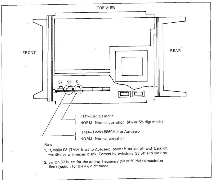
Figure 4-6. Slide Switches Used in Troubleshooting
