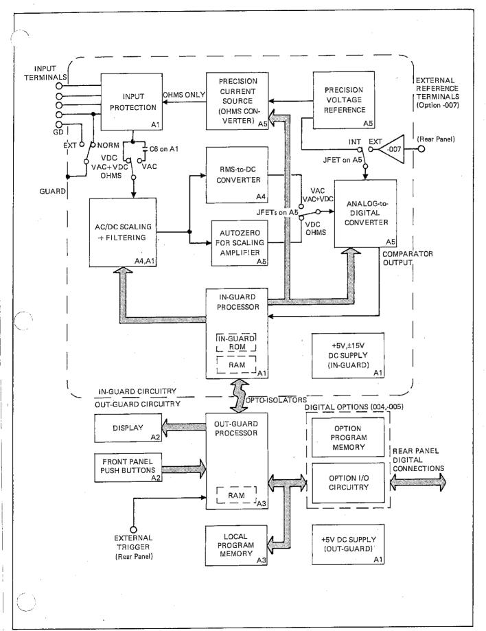
Figure 3-1, 8860A Block Diagram
