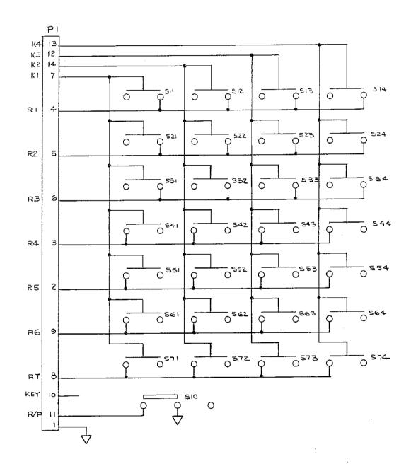
Figure 8-11. Control Keyboard PCB Assembly
