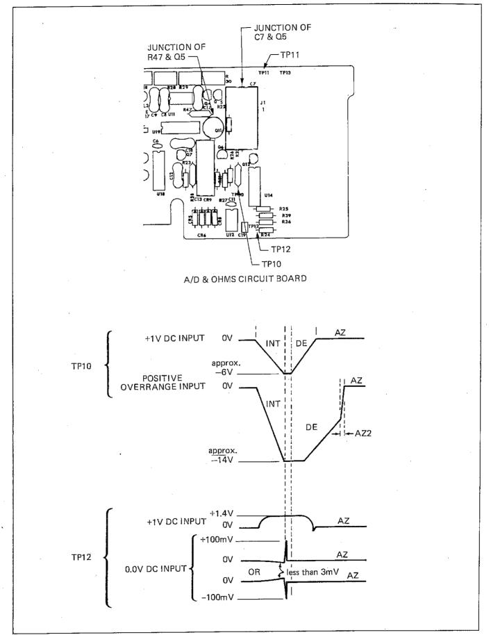
Figure 4-5. Signal Waveforms in A/D Converter (cont)
