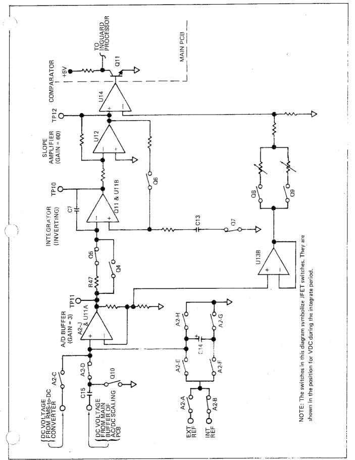
Figure 3-6. A/D Converter—Simplified Schematic
