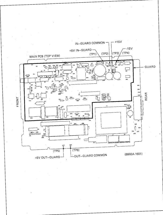
Figure 4-2. Power Supply Test Points
