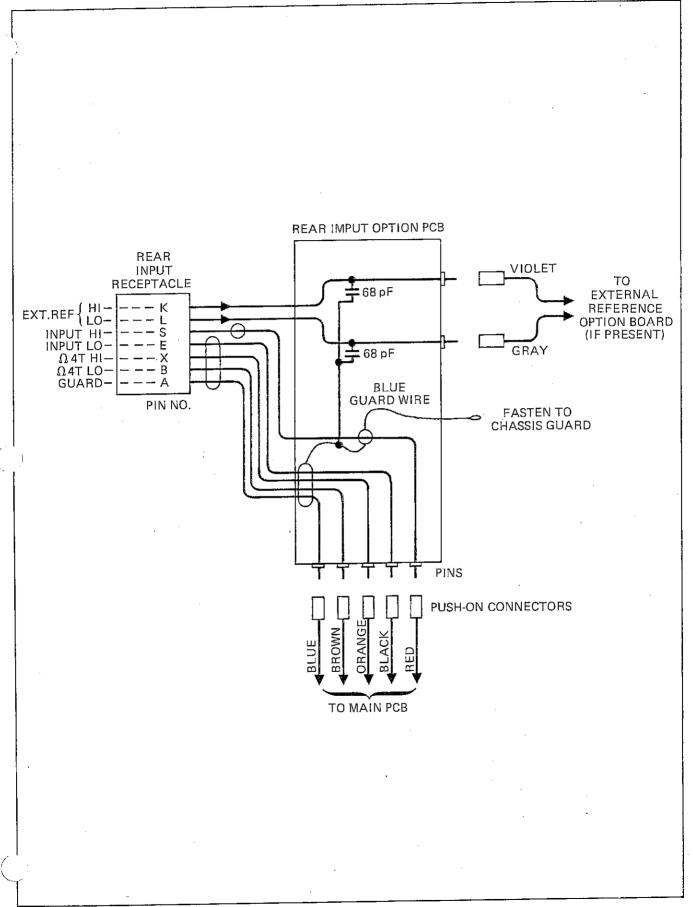
Figure 006-1. Rear Input Option Schematic
