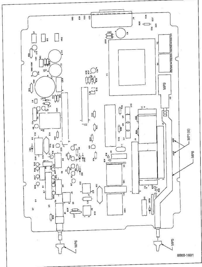
Figure 5-2. A1 Main PCB Assembly
