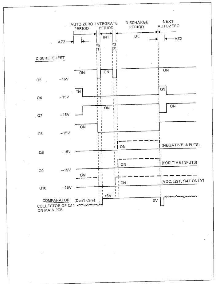
Figure 4-4. Timing Diagram for A/D Converter JFETs (cont)
