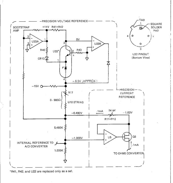
Figure 3-8. Precision Voltage and Current References—Simplified Schematic
