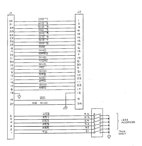
Figure 8-13. Rear Interconnect PCB Assembly
