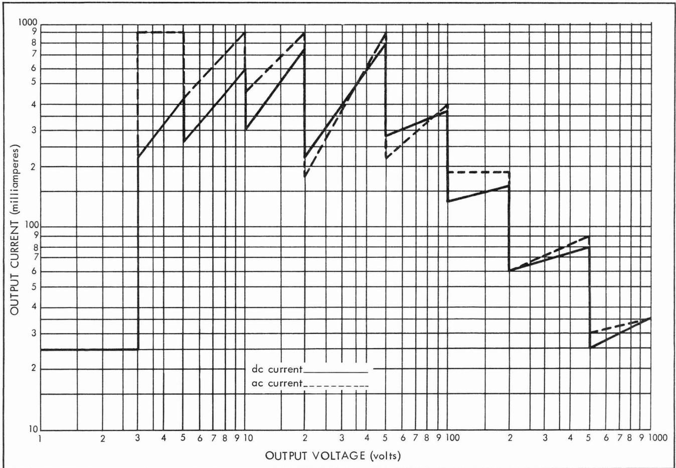
Figure 1-2. MAXIMUM OUTPUT LOAD CURRENT IN VOLTAGE MODE
