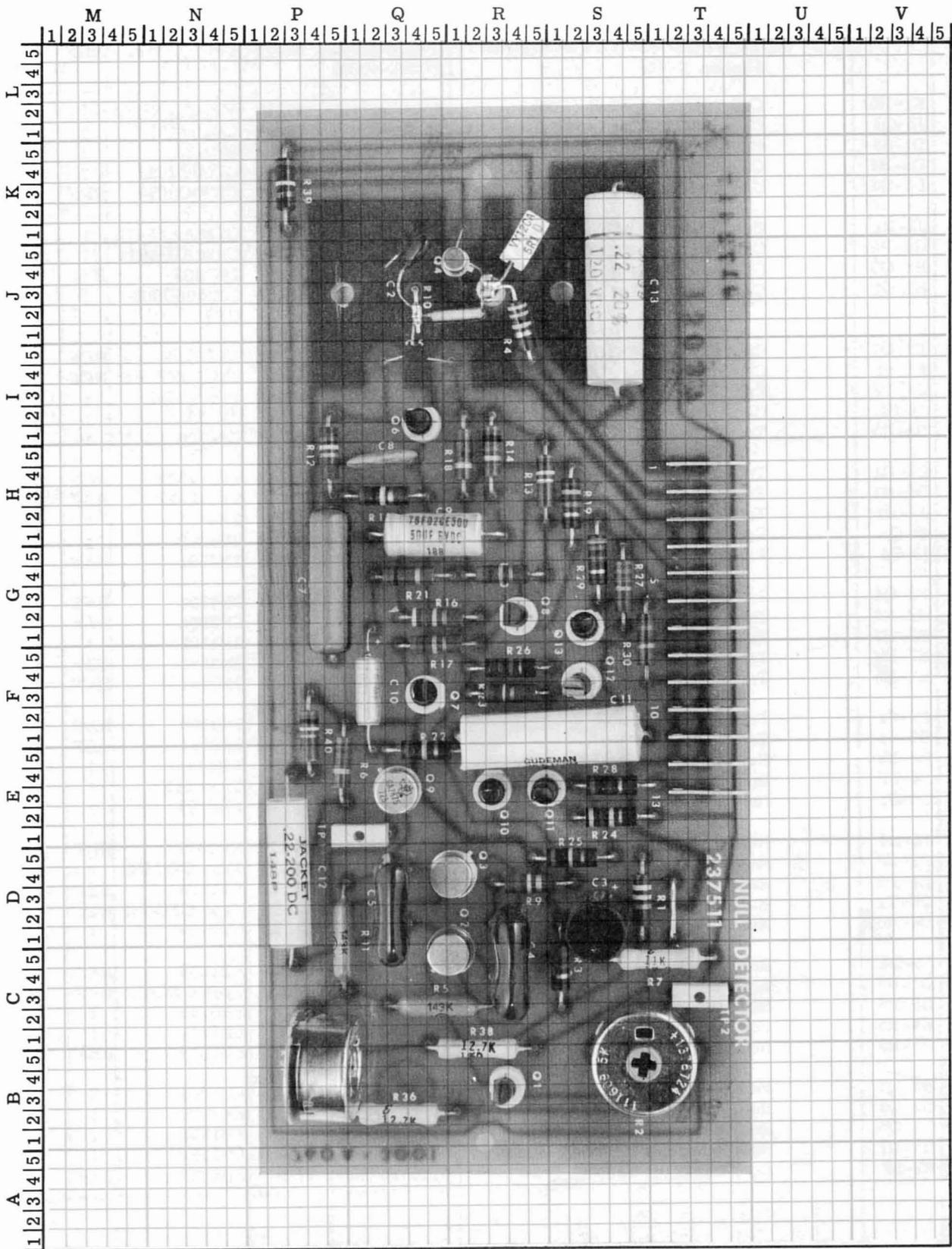
Figure 5-14. NULL DETECTOR P/C ASSEMBLY
