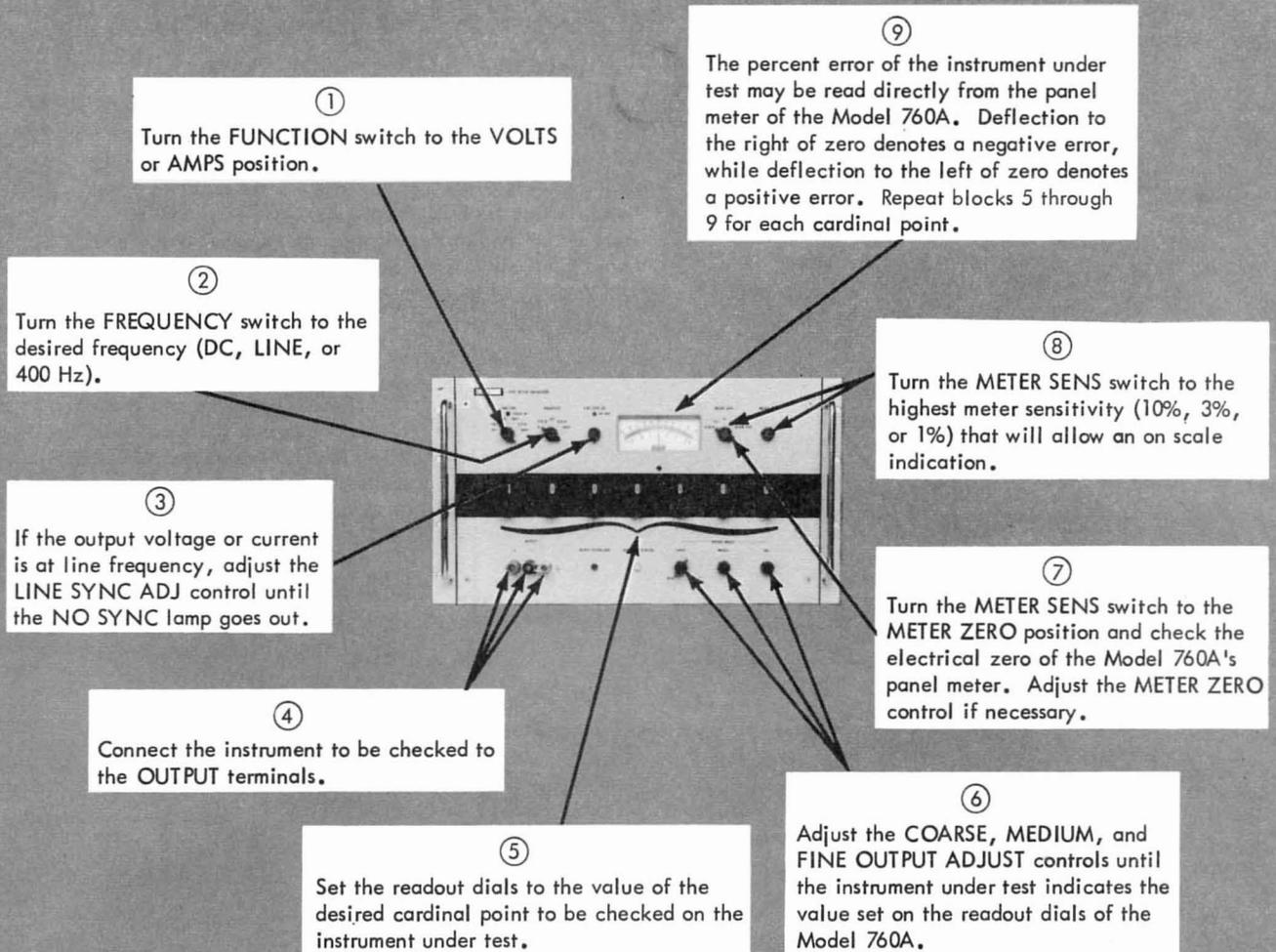
To determine the error in terms of voltage or current, follow instruction blocks 1 through 5 and substitute the following information for the remaining blocks:
