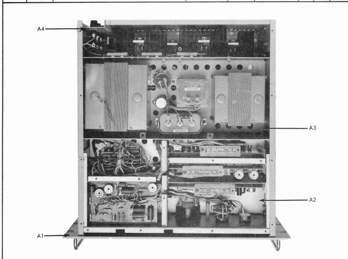
Figure 5-1. 760A METER CALIBRATOR
