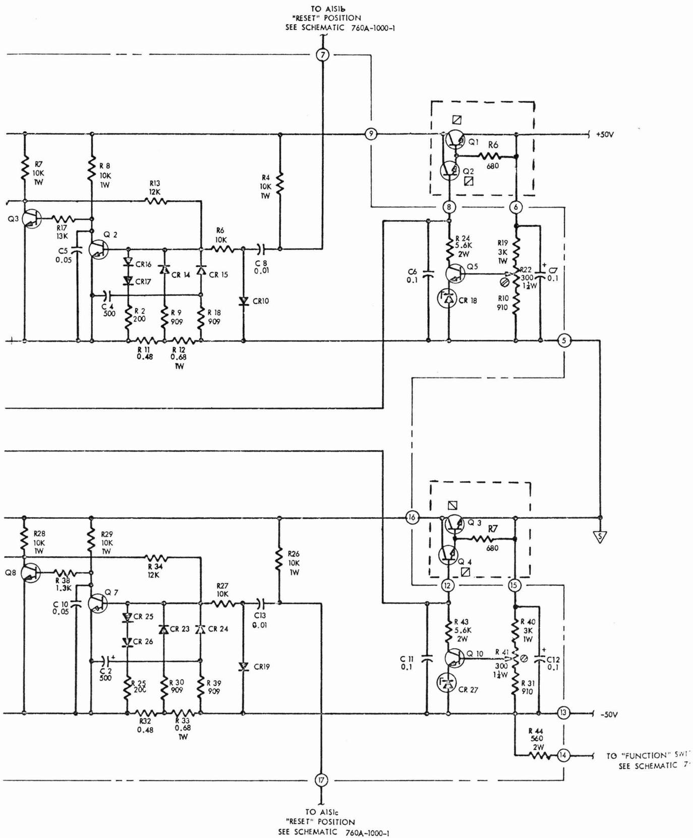
Figure A. LOCATION OF R6 AND R7 ON ±50 VOLT POWER SUPPLY SCHEMATIC
