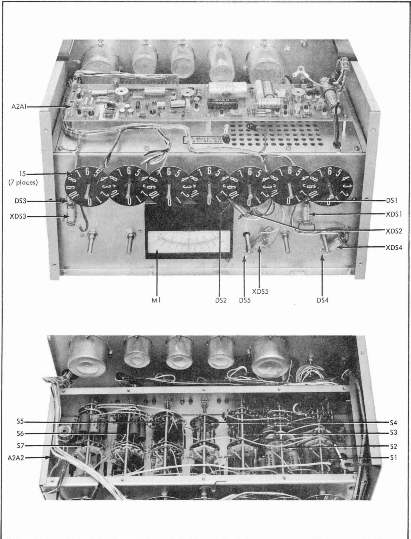
Figure 5-3. MEASUREMENT CHASSIS ASSEMBLY
