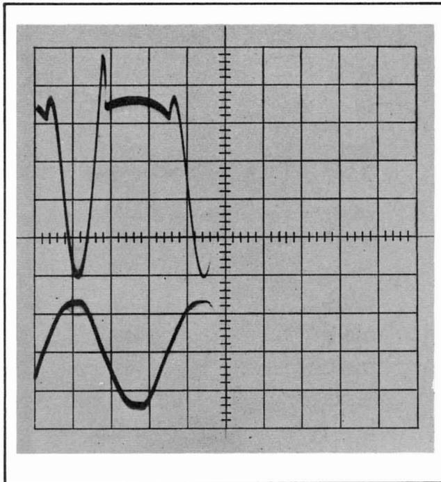
Figure 4-14. SYNCHRONIZING CIRCUIT INPUT AND OUTPUT WAVEFORMS WITH OSCILLATOR SYNCHRONIZED
