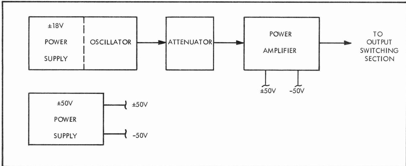
Figure 3-2. SOURCE SECTION BLOCK DIAGRAM
