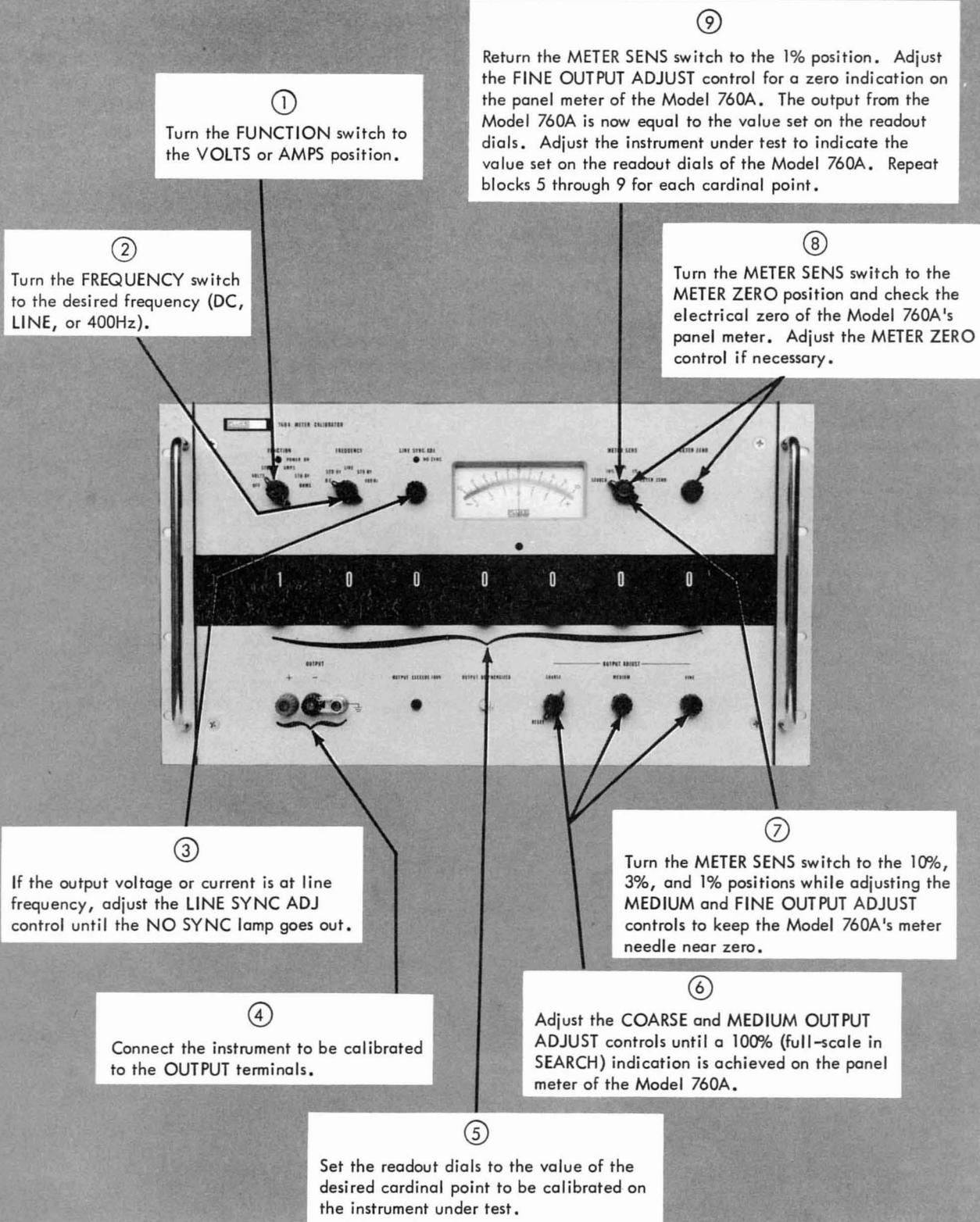
Figure 2-3. CALIBRATING A VOLTAGE OR CURRENT MEASURING INSTRUMENT
