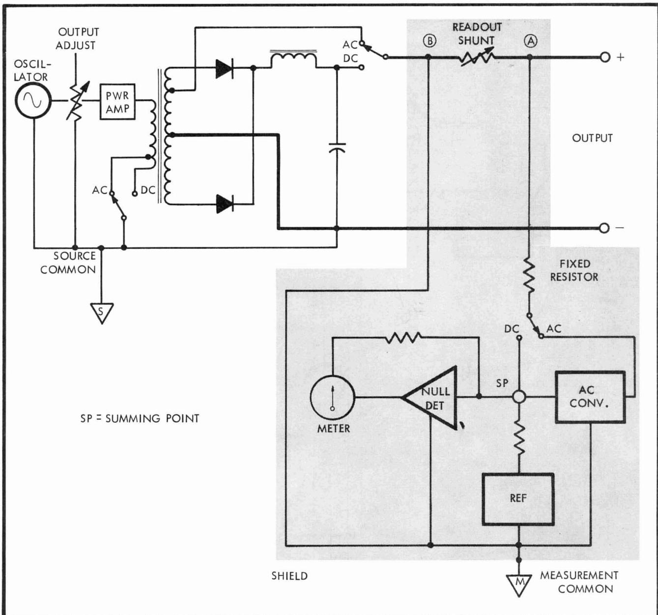
Figure 3-6. LOW CURRENT ARRANGEMENT
