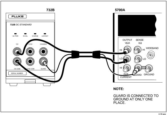
Figure 3-9. Typical 732B Cable Connections
