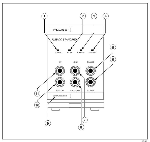
Figure 3-1. 732B DC Standard Front Panel Features
