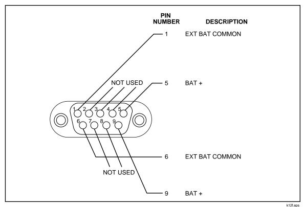
Figure 3-8. 732B-7001 BAT OUT Connector Pinout
