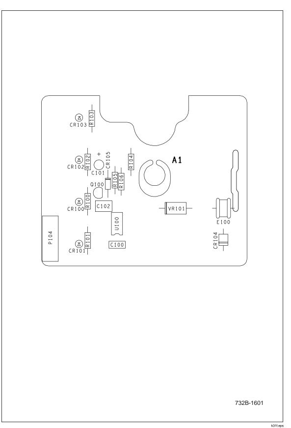
Figure 6-3. A1 Front Panel PCA
