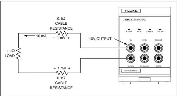
Figure 3-11. Loading Error Example
