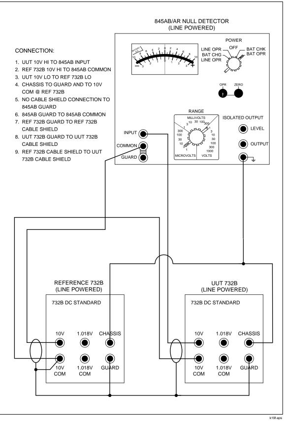
Figure 5-1. 10V Output Calibration Connections
