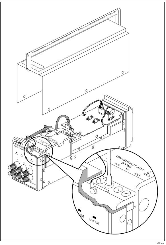
Figure 5-2. Location of 732B Calibration Adjustment Switches
