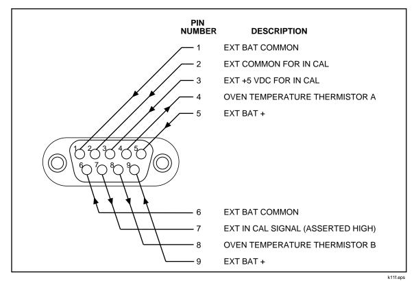
Figure 3-7. 732B MONITOR/EXT BAT IN Connector Pinout
