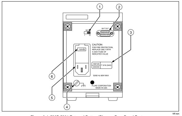
Figure 3-4. 732B-7001 External Battery/Charger Rear Panel Features
