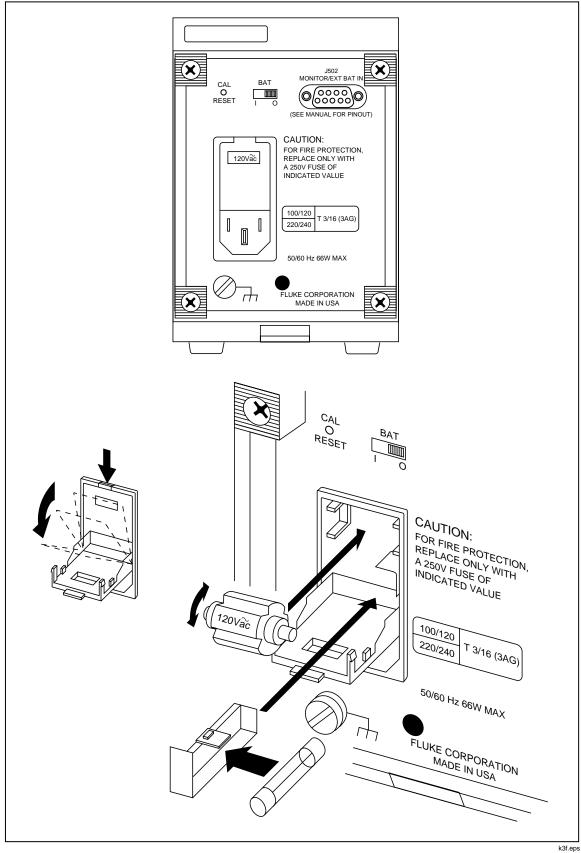
Figure 2-2. Line Power Label and Fuse Location
