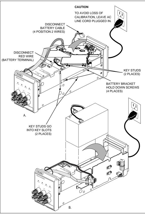
Figure 5-4. Replacing the Battery
