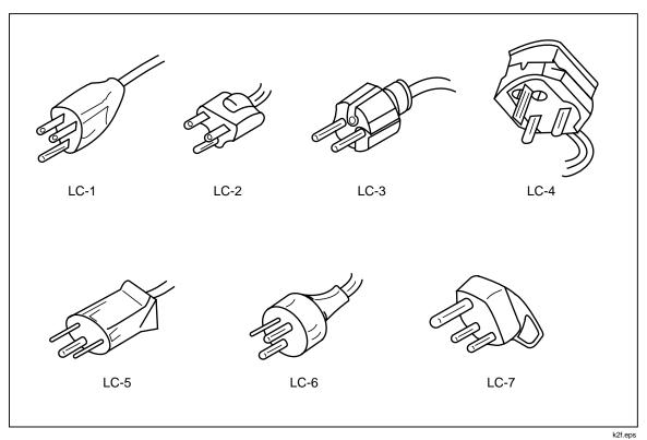
Figure 2-1. Line Power Cords Available for Fluke Instruments
