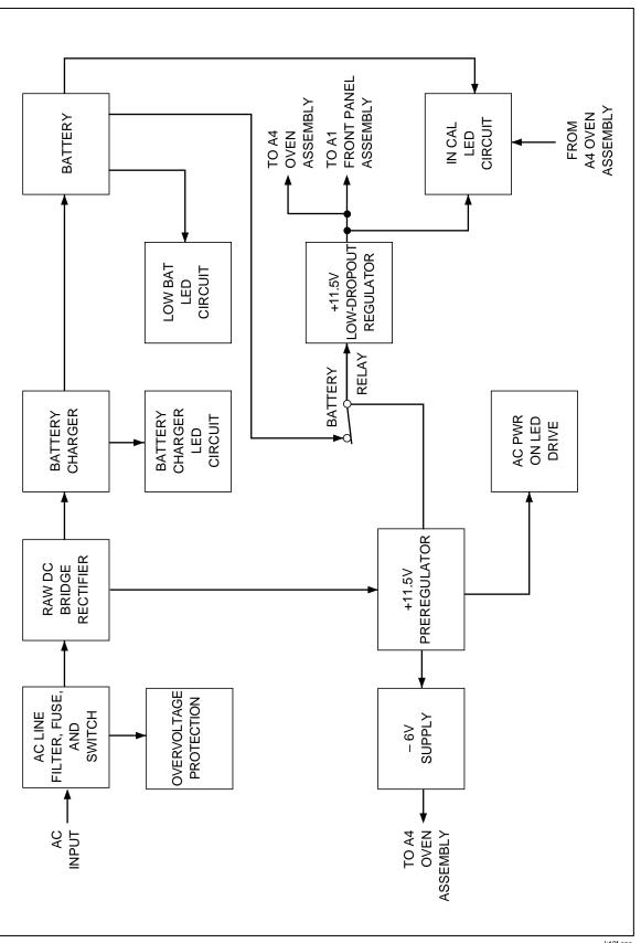
Figure 4-3. A5 Power Supply/Battery Charger Block Diagram
