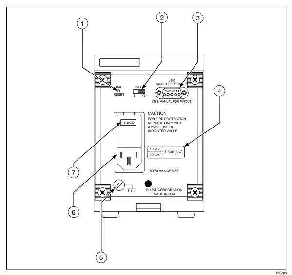
Figure 3-2. 732B DC Standard Rear Panel Features
