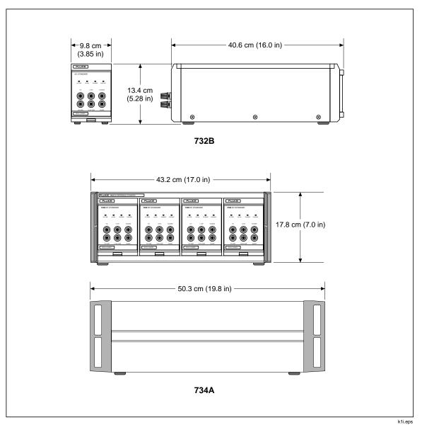
Figure 1-1. Mechanical Specifications
