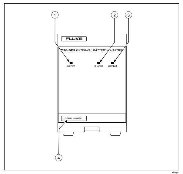
Figure 3-3. 732B-7001 External Battery/Charger Front Panel Features
