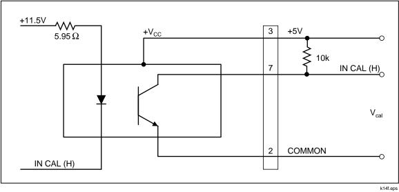
Figure 3-10. IN CAL Status Output Circuit
