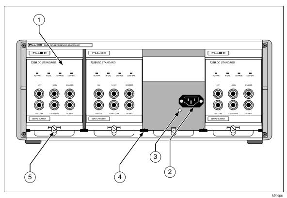
Figure 3-5. 734A-7001 Instrument Enclosure Front Panel Features
