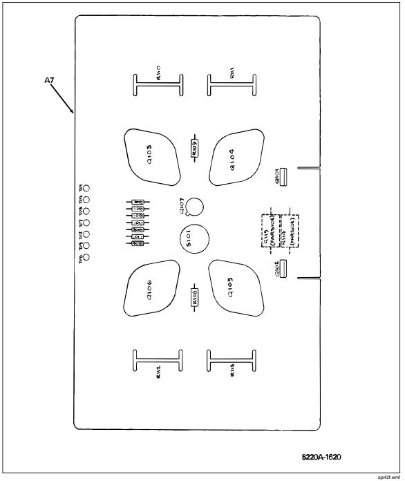
Figure 5-8. A7 Output PCB Assembly
