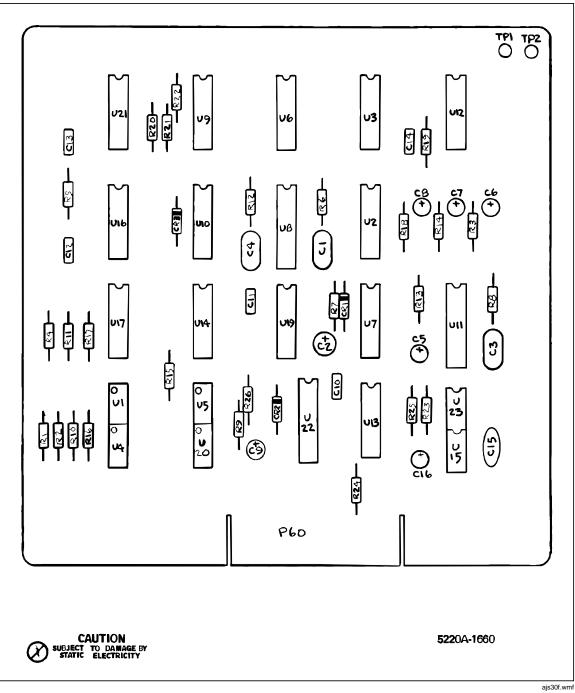
Figure 5-11. A10 Logic PCB Assembly
