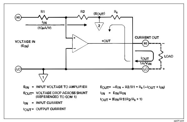
Figure 3-2. Transconductance Amplifier Simplified Circuit Diagram
