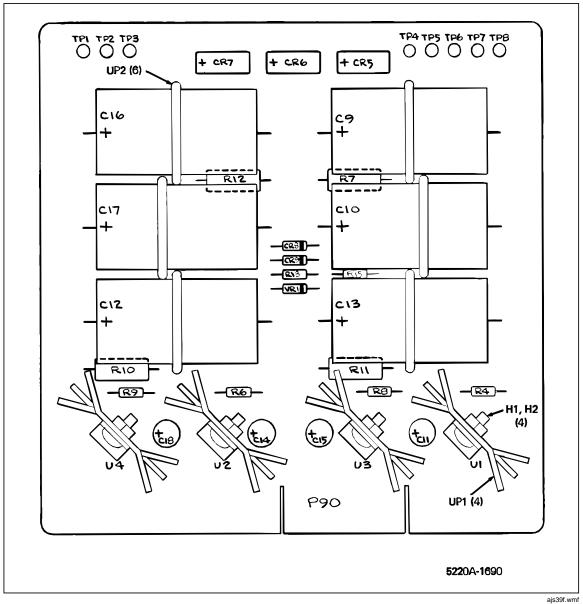
Figure 5-5. A4 Regulator PCB Assembly
