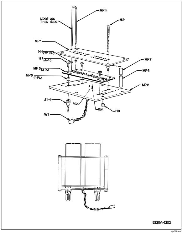
Figure 5-13. A12 Shunt Assembly
