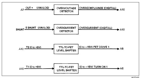
Figure 3-7. A8 Analog Control Simplified Block Diagram
