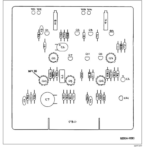
Figure 5-7. A6 Driver PCB Assembly
