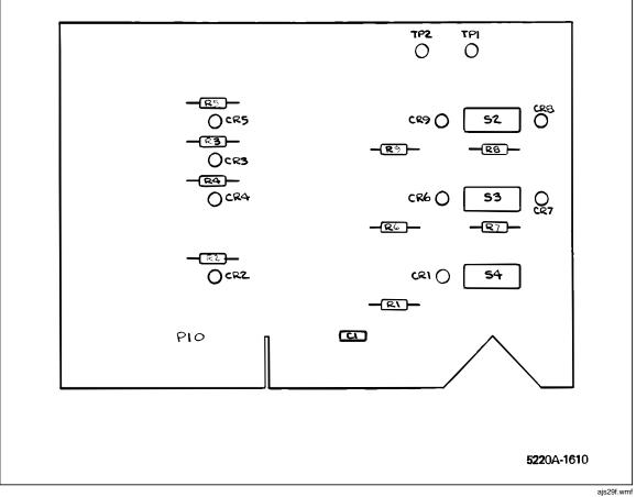
Figure 5-10. A9 Front Panel PCB Assembly
