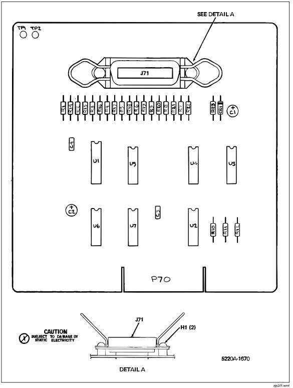
Figure 5-12. A11 MIS Bus PCB Assembly
