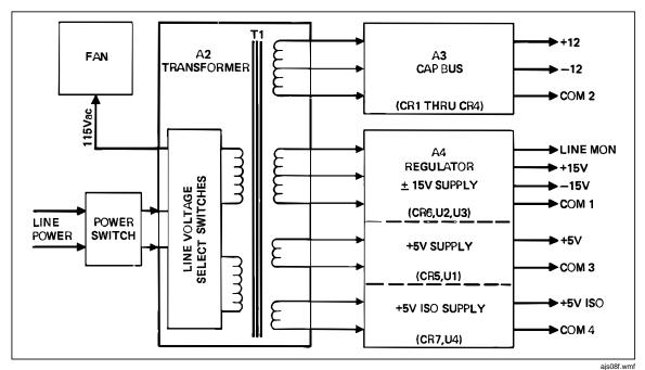
Figure 3-3. Power Supply Functional Block Diagram
