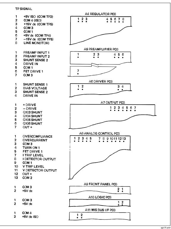
Figure 4-3. Test Point Location/Identification
