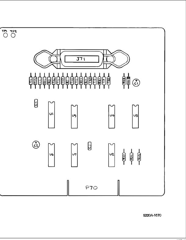
Figure 7-9. A11 MIS Bus Interface PCB Assembly
