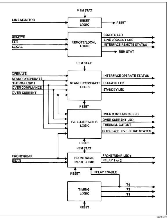
Figure 3-8. A10 Logic Simplified Block Diagram
