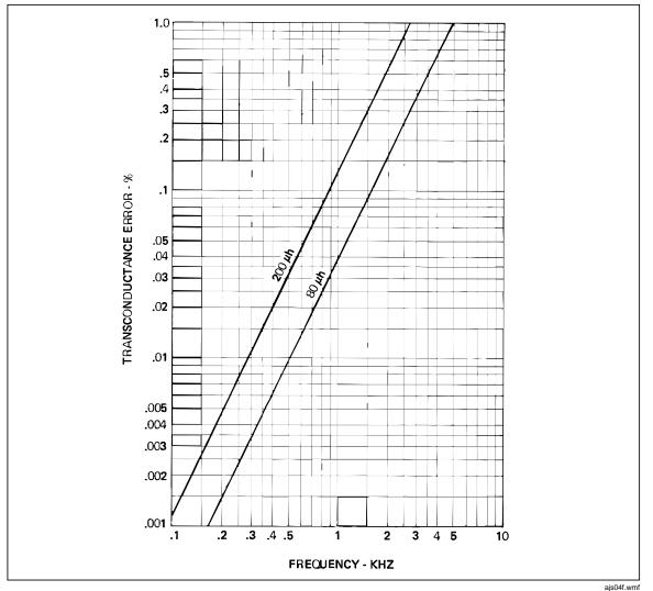
Figure 2-3. Typical Transconductance Error for Inductive Loads
