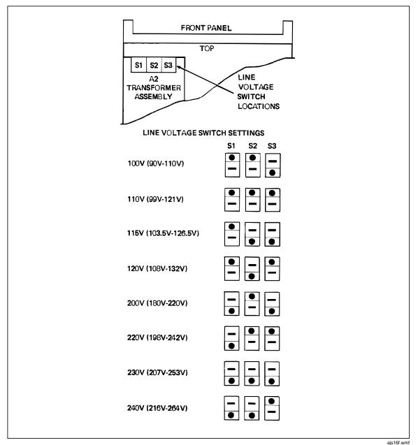
Figure 4-2. Line Voltage Selection
