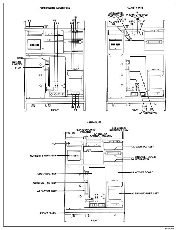
Figure 4-1. Internal Component/Assembly Locations
