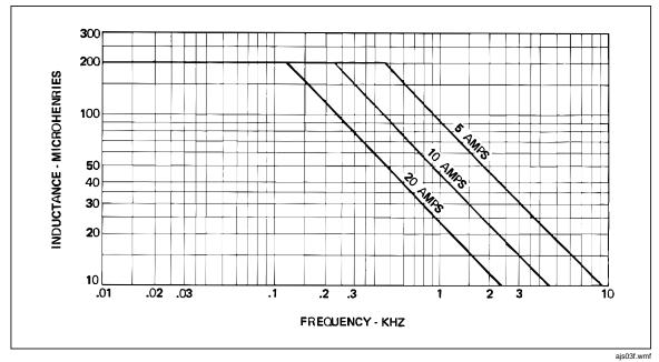
Figure 2-2. Maximum Load Inductance vs Frequency
