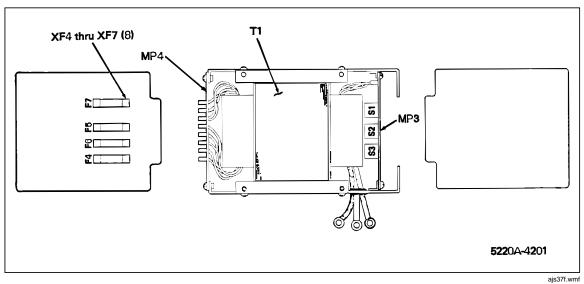
Figure 5-3. A2 Power Transformer Assembly
