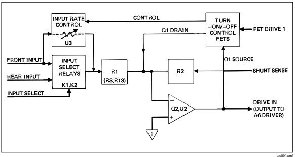
Figure 3-4. A5 Preamplifier Functional Block Diagram
