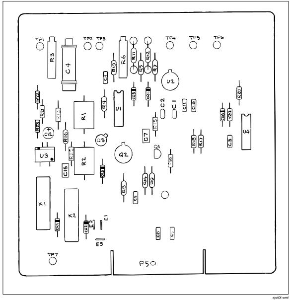
Figure 5-6. A5 Preamplifier PCB Assembly
