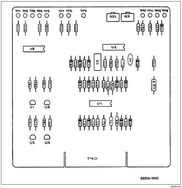
Figure 5-9. A8 Analog Control PCB Assembly
