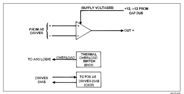
Figure 3-6. A7 Output Functional Block Diagram
