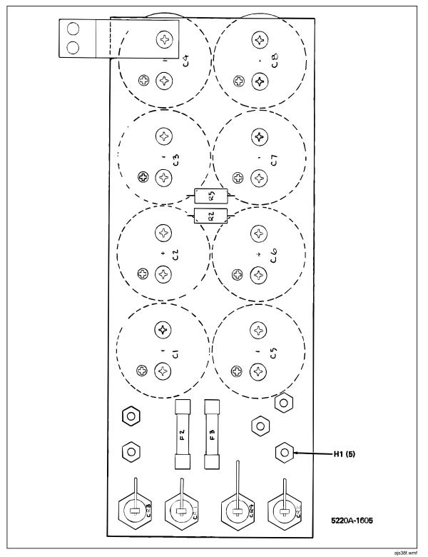
Figure 5-4. A3 Capacitor Bus PCB Assembly
