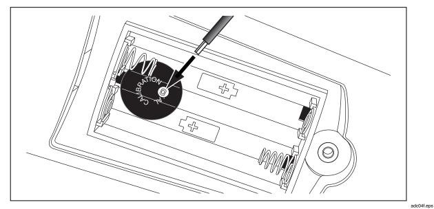
Figure 7. Calibration Adjustment (336-337)
