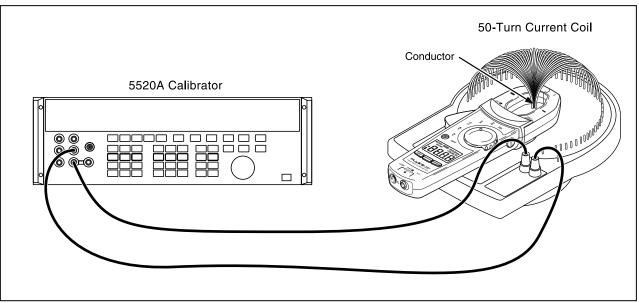
Figure 4. 33x Amps/Hz Verification Setup
