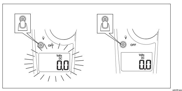
Figure 3. Testing the Backlight
