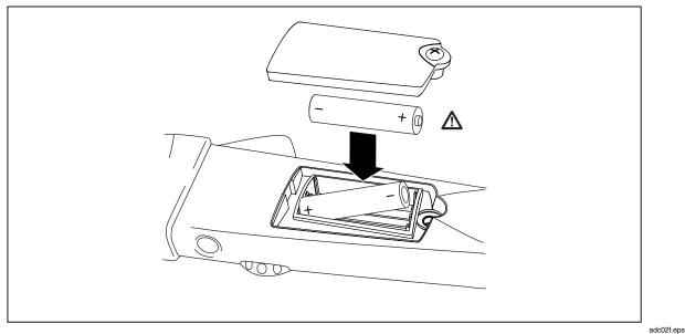
Figure 1. Replacing the Batteries
