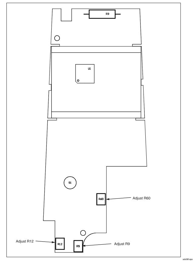
Figure 6. Calibration Adjustment Points 336-337
