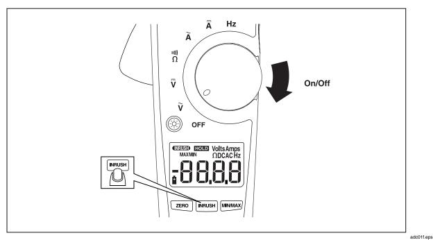
Figure 2. Testing the Display (337 is shown)
