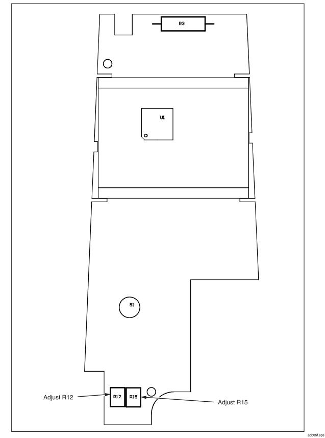
Figure 5. Calibration Adjustment Points (333-335)
