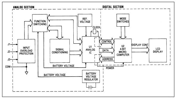
Figure 2-1. Overall Functional Block Diagram
