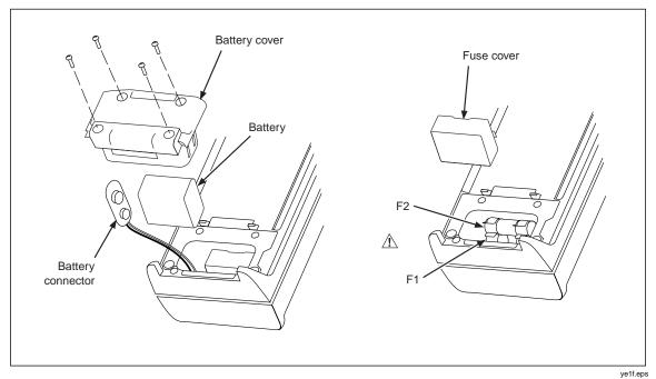
Figure 3-1. Battery and Fuse Replacement
