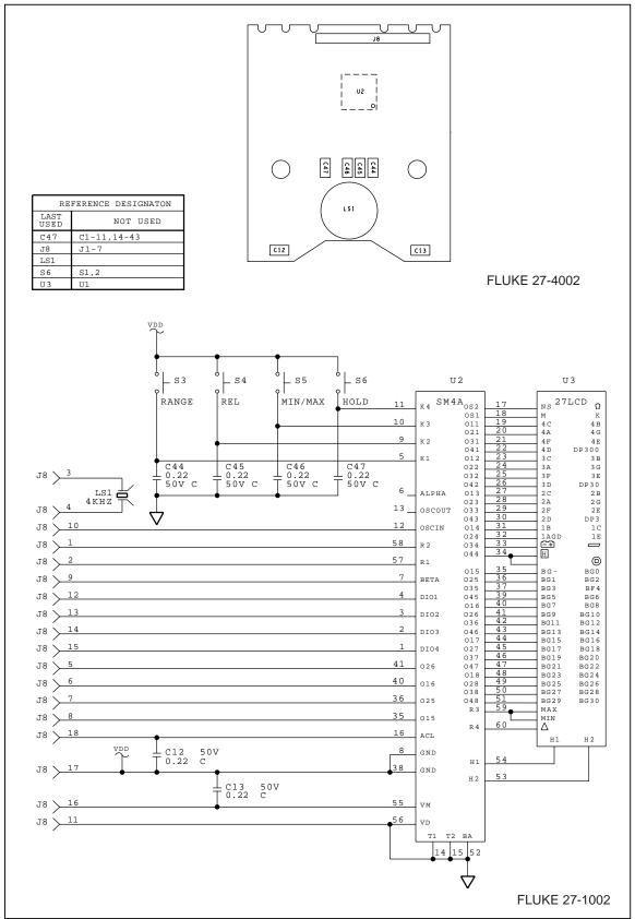
Figure 5-1. A1 Main PCA and A2 Digital PCA (cont)
