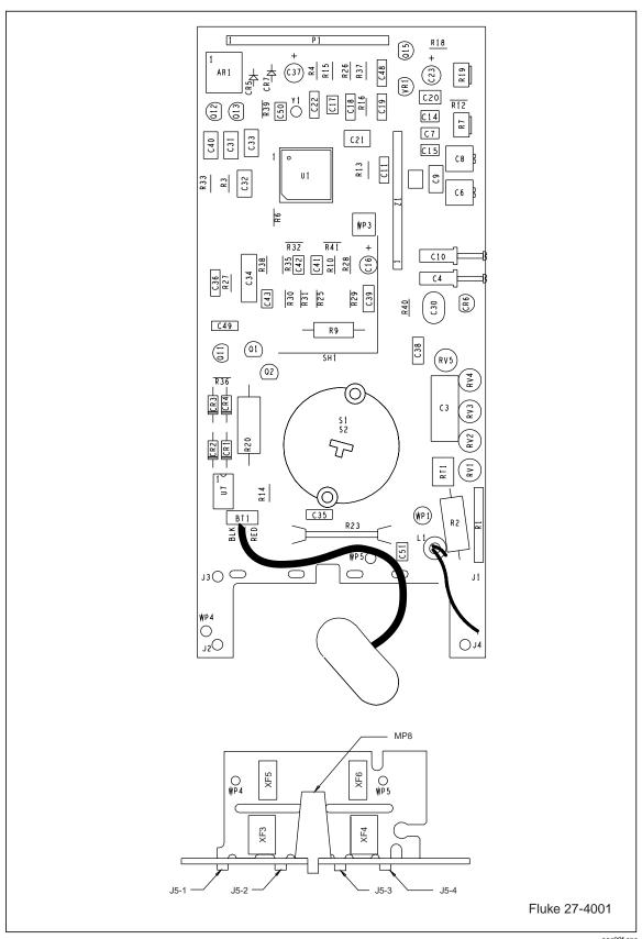
Figure 5-1. A1 Main PCA and A2 Digital PCA
