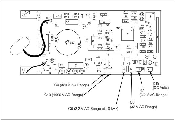
Figure 3-3. Calibration Adjustment Locations
