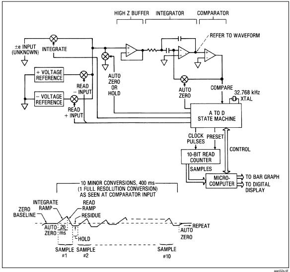
Figure 2-2. A/D Conversion Elements and Waveform
