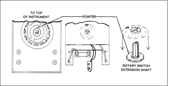
Figure 3-3. Switch Extension Shaft Installation
