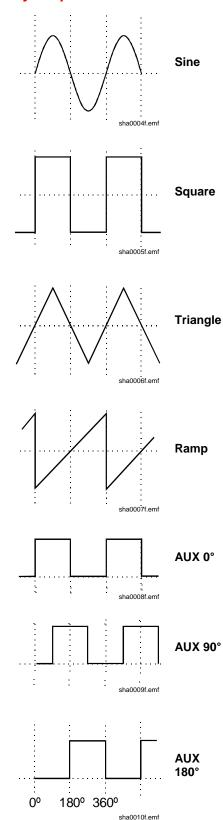
The convention adopted for phase in this instrument is illustrated in the diagram.  $0^{\circ}$  is always the first data point in waveform memory. On symmetrical waveforms  $0^{\circ}$  is the rising edge zero-crossing point for sine, square, triangle and pulse waveforms; on ramps, staircases and arbitrary waveforms  $0^{\circ}$  is always the start point.
