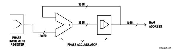
On each clock cycle the phase increment, which has been loaded into the phase increment register by the CPU, is added to the current result in the phase accumulator; the 10 most significant bits of the phase accumulator drive the RAM address lines. The output waveform frequency is now determined by the size of the phase increment at each clock. If each increment is the same size then the output frequency is constant; if it changes, the output frequency changes but with phase continuity.
