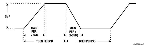
Set the main generator to 10 kHz, 10 V p-p, by pressing **FREQ**, **1**, **0**, **kHz**, and **VhiZ**, **1**, **0**, **V**; change the symmetry to 60:40 by pressing **SYM**, **6**, **0**, **%**; **DC OFFSET**, **0**, **V**; select **TRIANGLE**.
