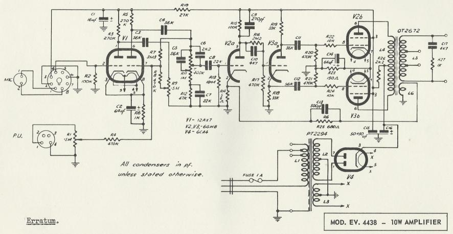
Volume control is tapped at 100K not 400K, as shown on circuit drawing.
