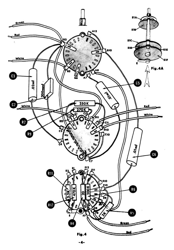
The following instructions cover the prewiring of the range switch, S1, as shown in Fig. 4. To see the switch as shown in Fig. 4, hold it with the shaft pointing away from you and with the ground lug E on the under side. Fig. 4 A is a perspective drawing of switch, S1, indicating the view employed in Fig. 4.
