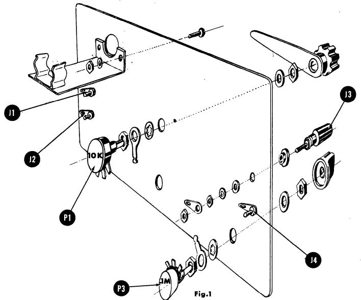
Fig. 1. Mount the four binding posts, J1-J4 as shown. Use one #8 fibre shoulder washer, one #8 flat fibre washer, one #8 solder lug, and two 8-32 hex nuts in mounting each.
