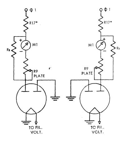
k) MERIT TEST for power rectifier section A of full-wave type.
