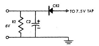
TRANSISTOR TEST POWER SUPPLY
