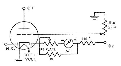
i) MERIT TEST of light-duty diodes, (showing one diode section of a triode duo-diode, such as a 12SQ7).
