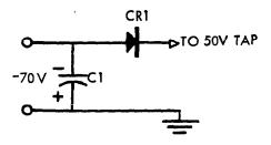
LEAKAGE TEST POWER SUPPLY — Also used for Line Adjust.
