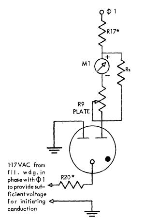
j) MERIT TESTING of OZ4, OY4 cold-cathode gas rectifiers (test of one section of OZ4 shawn).
