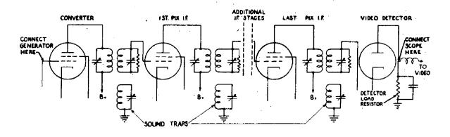
TYPICAL TELEVISION INTERMEDIATE FREQUENCY AMPLIFIER AND DETECTOR
