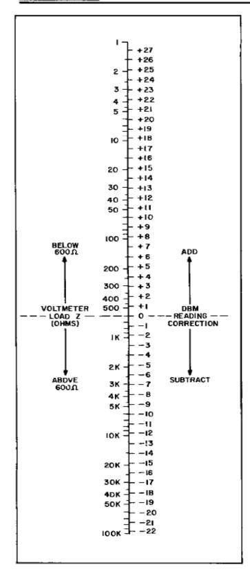
Figure 2-2. Nomograph of DB Connections vs. Load Impedance for DBM Readings in Voitmeter Operation.
