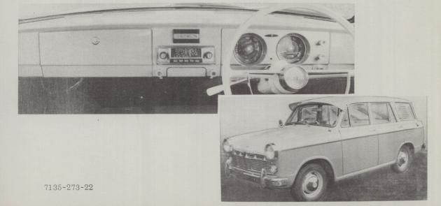
THE RECEIVER is to be mounted behind the instrument panel at a position occupied by an oblong cover panel. A rear bracket supports the passenger side corner to top underside of panel.
