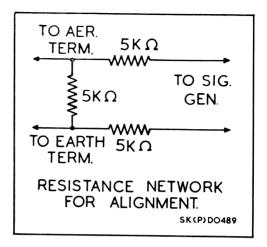
Note: Non-inductive resistors should be used in the above network. Sensitivity figures obtained will not represent the true sensitivity of the instrument; purpose of the network is to obtain optimum alignment of the loop when used without an external aerial.
