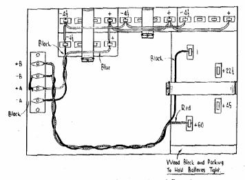
Fig. 1.-Installation and Connection of Batteries.
