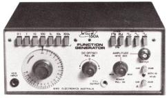
The BWD160A is a very moderately priced generator providing 12 different waveforms and 5 simultaneous outputs. It can be swept over any section of its frequency range up to 4 decades wide by the BWD170 log or linear ramp output. Pulse or ramp outputs of either polarity have a fixed mark-space ratio of approx 20–1 thus maintaining a constant calibration at 1/10th the indicated
