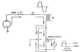
Figure 3. Diode and Rectifier Emission Test
