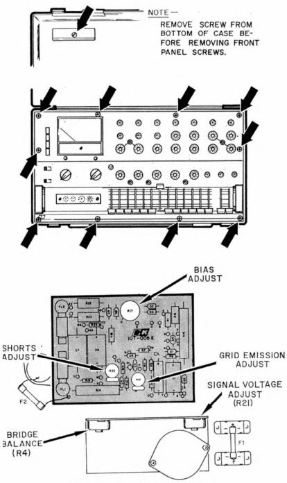
Figure 12. Parts and Adjustment Locations
