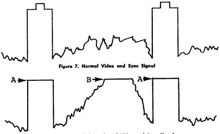
Figure 8. Overloaded or Clipped Video and Sync Signal
