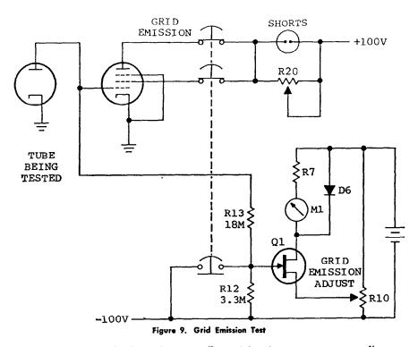
Q1. This FET is also biased to cut-off, resulting in a zero meter reading.
