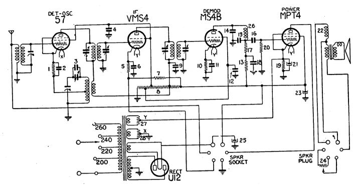
Genalex model "BC200" is a five-valve receiver designed for broadcast coverage and operation from 200-260 v. A.C. mains. This receiver is fitted to a compact mantel type cabinet and is fitted with two controls, these being for tuning and volume. This model was marketed during 1935.
