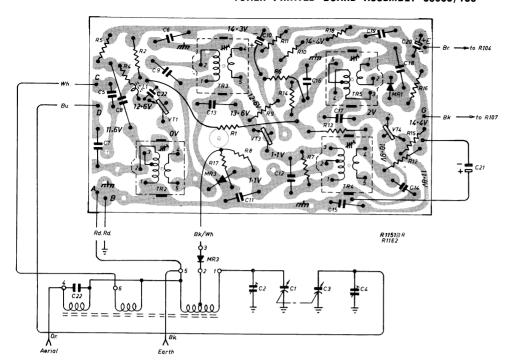
Notes: The diagram represents the view from the wiring side of the printed board.
