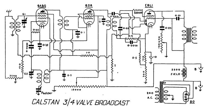
Calstan model "B4M" is a four-valve receiver designed for broadcast coverage and operation from 200-260 v. A.C. mains. This receiver is of the mantel type, and although normally fitted with only two controls (volume and tuning), is sometimes equipped with a continuously-operating tone control, wired across the output valve plate as shown in the diagram. The loudspeaker fitted to this receiver is a 61-inch diameter unit with a field-coil resistance of 2.500 ohms.
