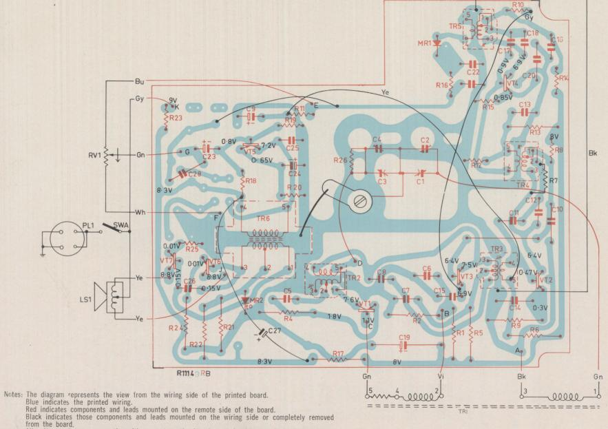
All voltages shown are negative with respect to the board earth (positive terminal of the battery) and measured with no signal input and volume maximum clockwise using a 20,000 ohm/volt meter.
