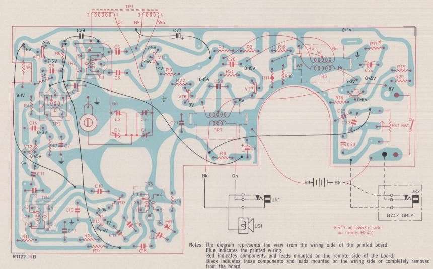
All voltages shown are negative with respect to the board earth (positive terminal of the battery) and measured with no signal input and volume maximum clockwise using a 20,000 ohm/volt meter.
